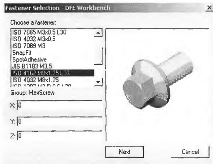
Figure 3.29 The DFE Workbench fastener selection window in SolidWorks 2000
