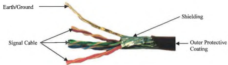
Figure A.4 Image of a DAQ cable which highlights the presence of Shielding [Source: www.ni.com , 2008].
