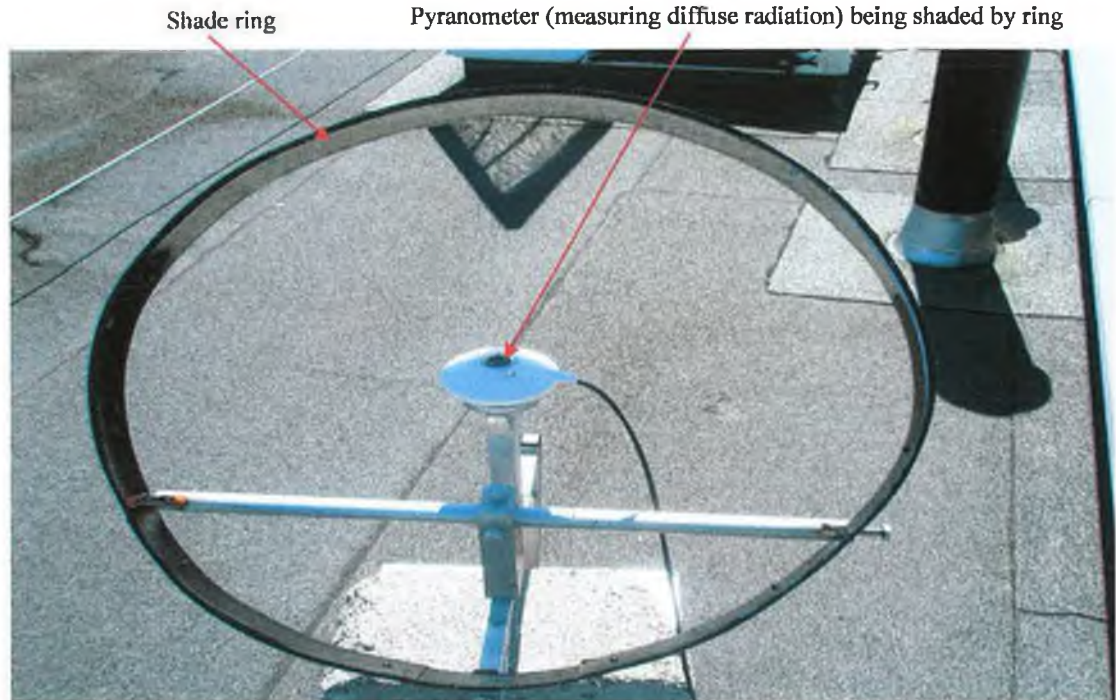
Figure 3.3 Photograph of the pyranometer measuring shortwave diffuse radiation fitted with a shade ring positioned on the liBC building's plant room roof.
