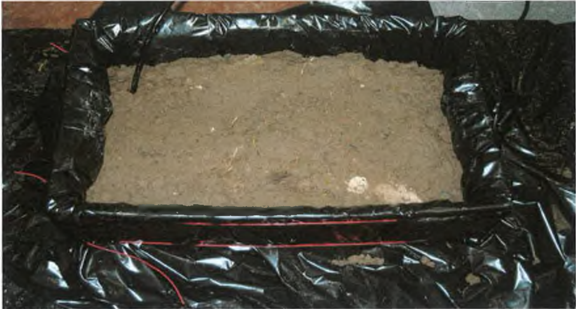
Figure A.7 Photograph of the Moisture sensor immersed in a sample of soil only for calibration.
