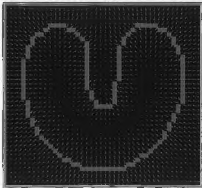
Figure 4.8.1.1: A gradient vector flow (GVF) field for a U-shaped object. These vectors will pull an active contour toward the boundary of the object.
