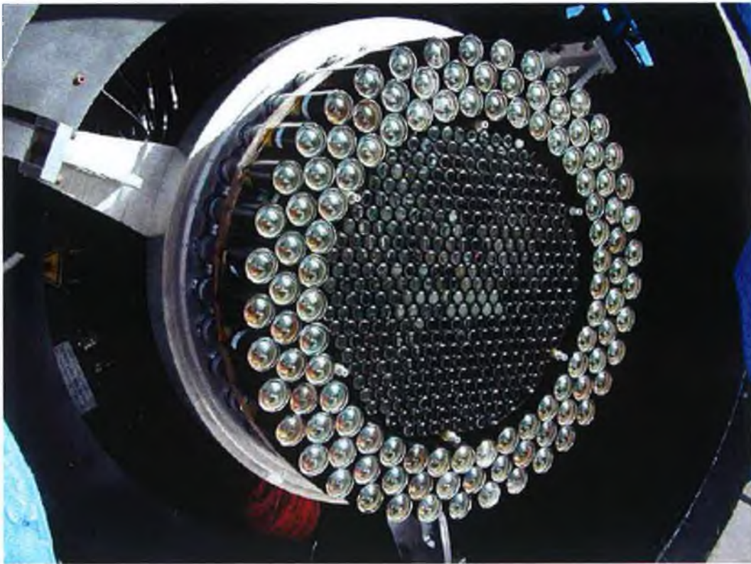
Figure 3.3: The 490-PMT camera used in the Whipple 10m telescope from 1999 to 2003. The outer 111 PMTs were removed in January 2003 to be used as part of the VERITAS prototype telescope. Image taken from http://veritas.sao.arizona.edu/old/Photos/G3Camera2.html
