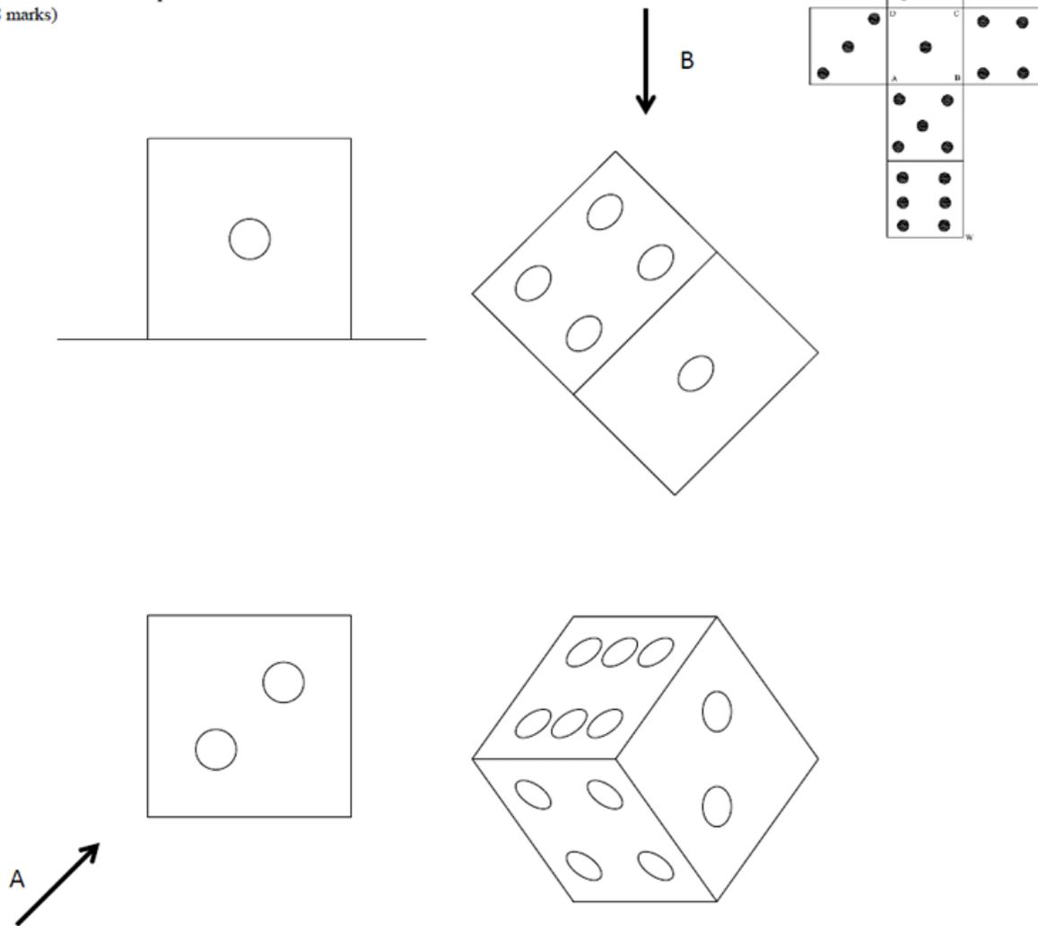
Figure 2. Solution to graphical problem posed to participants. The solution required producing the first and second auxiliary views in the directions of arrows A and B respectively. Performance was evaluated based on correct orientation of the cube and positioning of the dice detail, not on quality of the presentation.
