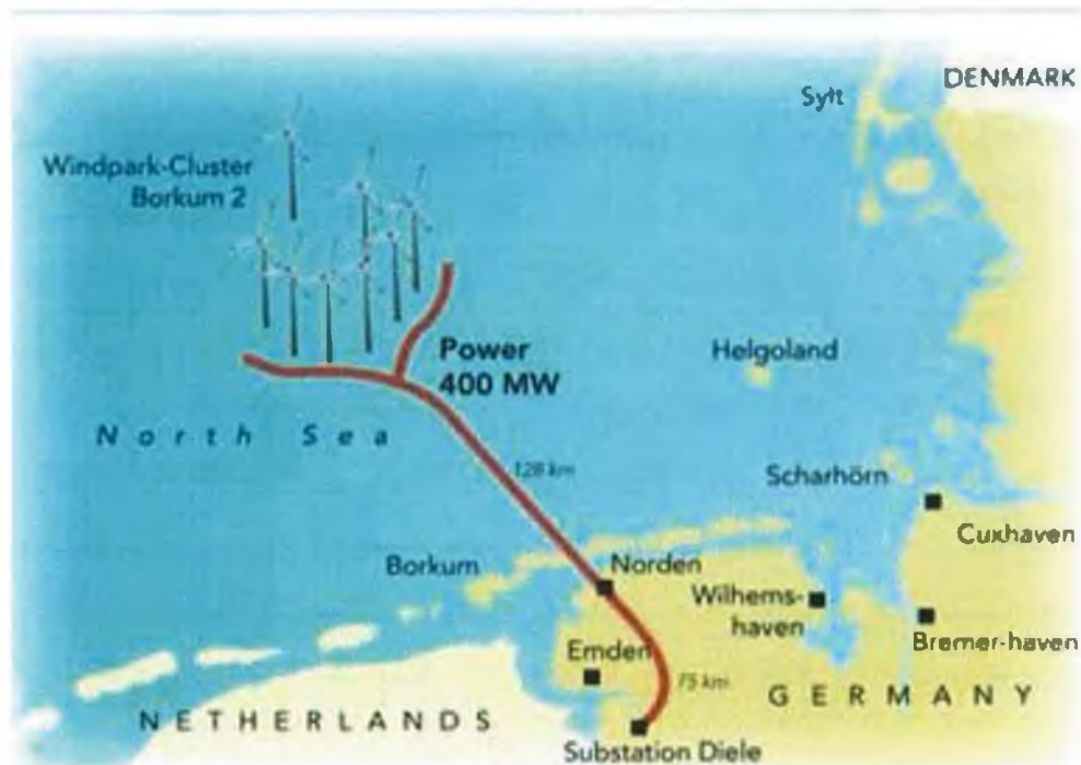
Figure 2.24 Offshore Windpark – Cluster Borkum (Gross, 2011)
