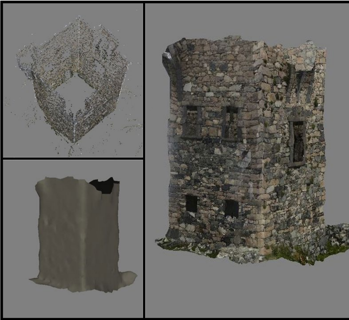
Figure 3.15. Generating a 3D model from overlapping photographs in PhotoScan. A selection of photographs were uploaded and used to generate a point cloud (top left). A simple mesh texture is then added to the point cloud (bottom left). Finally, the photographs are used to drape a realistic texture over the mesh (right).
