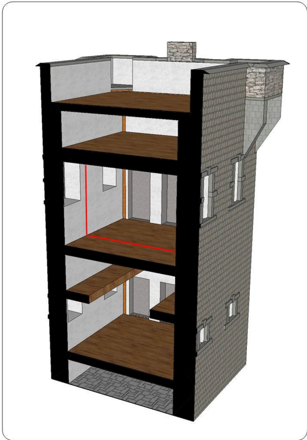
Figure 4.19. Rendered cut away version of the 3D model for an idealised tower showing the internal floors with the front wall removed, viewed obliquely. The red lines indicate a possible location of a dividing wall that separated the first-floor into two spaces.
