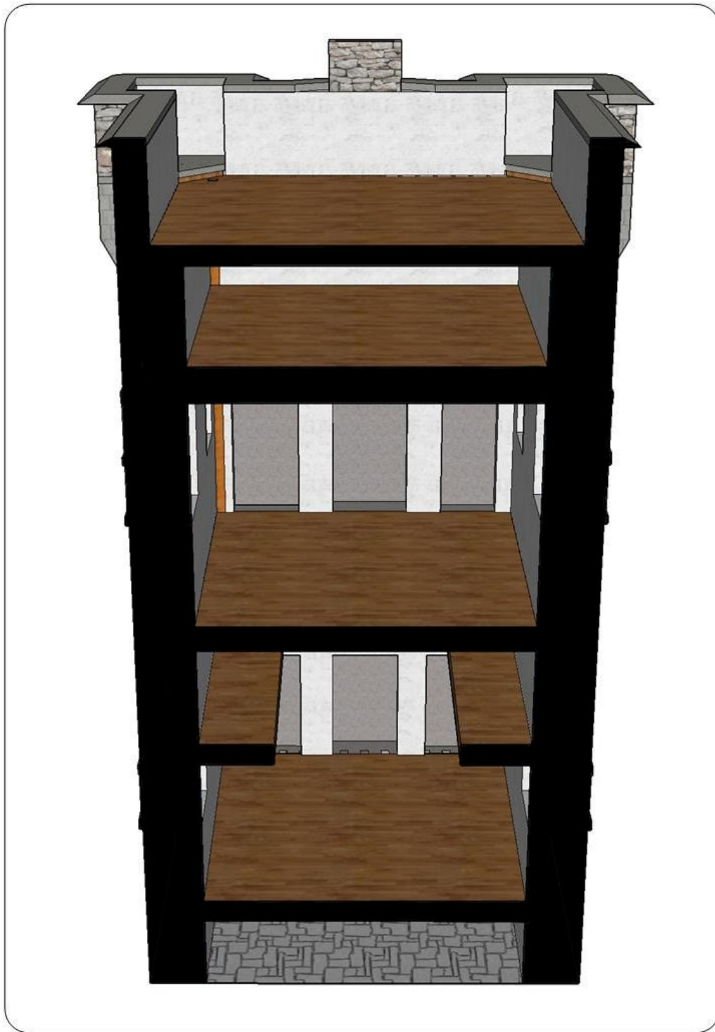
Figure 4.20. Rendered cut away version of the 3D model for an idealised tower showing the internal floors with the front wall removed, viewed square on.
