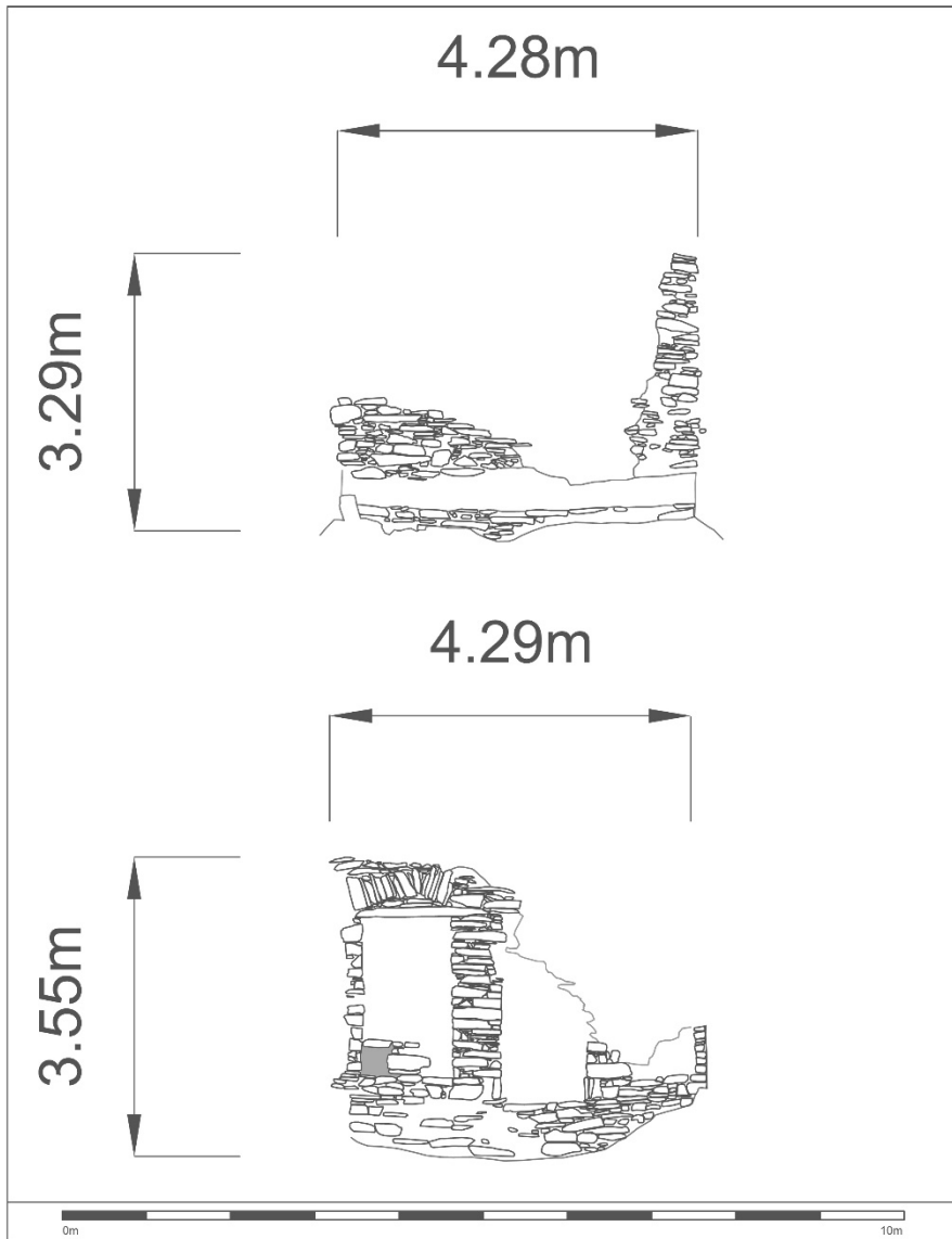
Figure B.15. Internal elevations of the south (top) and east (bottom) walls of Inishturk Signal Tower. The chute entering at the base of the ground floor alcove is shaded grey.
