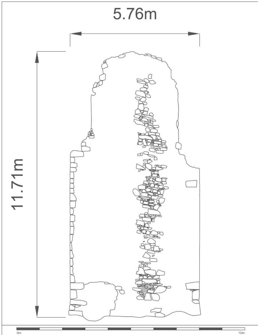
Figure D.76. External elevation of the south-east wall of the signal tower at Mullaghderg Hill Signal Tower.
