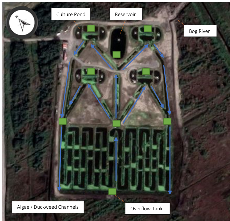
Fig. 1. Aerial view of Oasis Fish Farm, located in Ballycon, Co. Offaly. The culture ponds, water reservoir, algae & duckweed wastewater treatment channels, overflow tank and bog river are all visible. Blue lines indicate the direction of the flow of water. The green squares indicate all sampling points within the farm to monitor the IMTA process.
