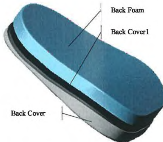
Figure 6.6. The CAD representation of the Back Assembly
