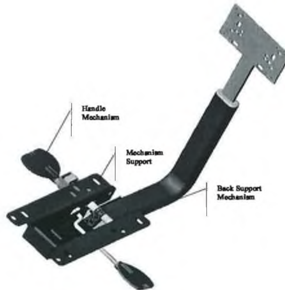
Figure 6.7. CAD representation of the Chair Mechanism
