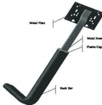
Figure 6.10. CAD representation of the Back Support Mechanism
