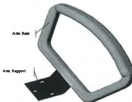
Figure 6.14. CAD representation of the Arm Assembly.
