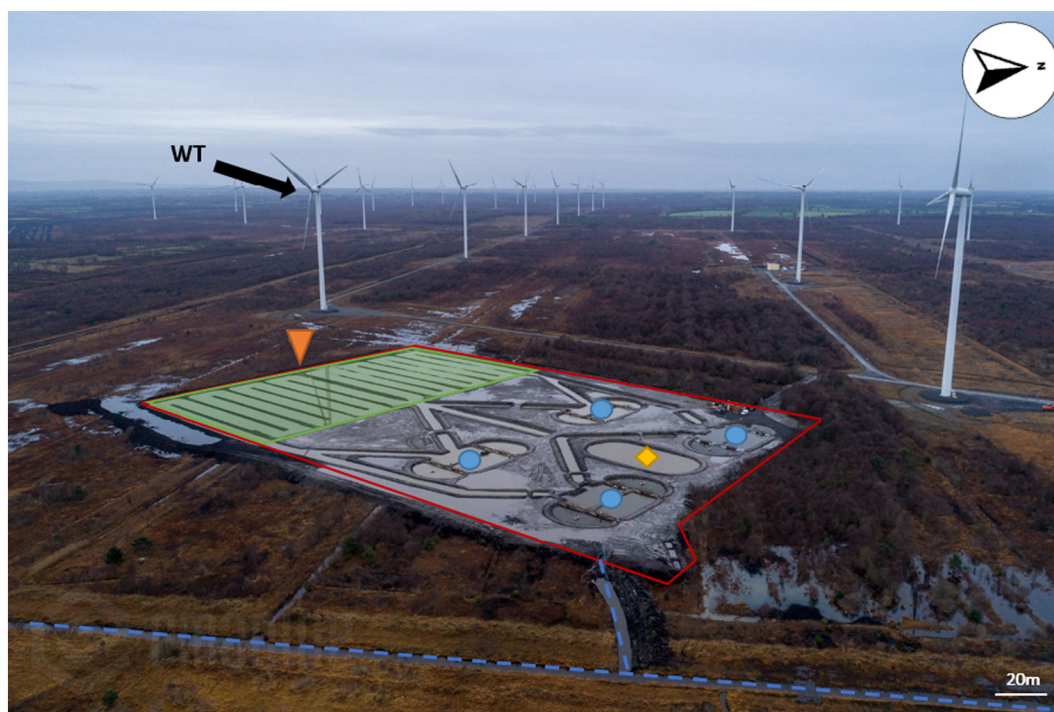
Fig. 1. Aerial view of Mount Lucas peatland site in the Republic of Ireland for development of aquatic innovations powered by wind turbines. The wind turbine indicated (WT) provides all electrical requirements for the production site (red). The site consists of 4 D-end split culture ponds (blue), a 16-channel treatment lagoon (green) which contains algae and duckweed, and a water reservoir (yellow) for the system. Water is taken from an adjacent bog river (---). This occurs only to compensate for loss of water from the system via evaporation. Discharge from the system only occurs during times of excessive rainfall whereby filling the overflow tank (orange). The site is situated in the middle of a peatland which is undergoing natural restoration.
