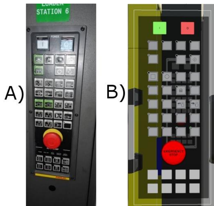
Figure 3.8: A) Real control panel on the Fanuc machine panel and B) VR panel developed within the virtual environment
