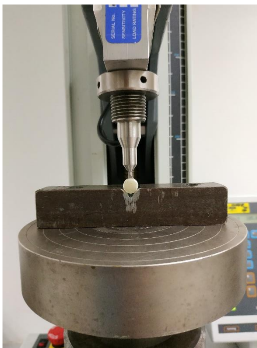
Figure 2.5 Set up for testing the interlayer adhesion force between inject moulded matrix and 3D printed substrates. The indentation on the aluminium block is 2.5 cm in depth on a straight angle.
