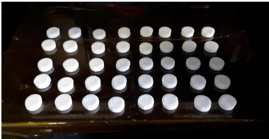
Figure 3.8 Complete batch of flat-faced tablets produced via FFF 3D printing. Total of 40 tablets covered print bed of MakerBot Replicator 2X.
