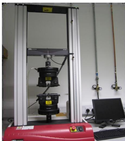
Figure 2-13: Instron tensile tester used in this study.
