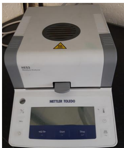
Figure 2-14: Mettler Toledo moisture analyser used in this study.
