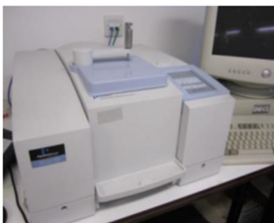
Figure 2-10: Perkin Elmer Spectrum One ATR-FTIR used in this study (left-hand side) and schematic diagram of FTIR (right-hand side).
