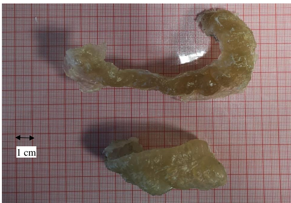
Figure 3-43: Typical appearance of extruded PNVCL samples after modifying the temperature (Profile 3) and screw speed (20 RPM).
