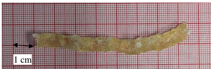
Figure 3-47: PNVCL sample processed using Temperature Profile 3 and a screw speed of 20 RPM, with the reduced moisture content and particle size.
