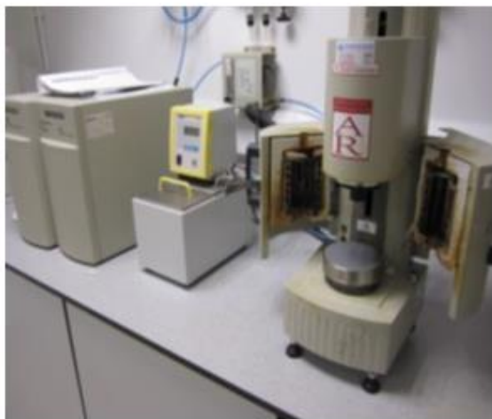
Figure 2-12: Advanced Rheometer AR 1000 (left) used in this study and schematic diagram typical for rheometry (right).
