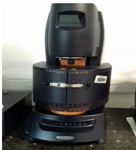
Figure 2-11: Discovery Hybrid Rheometer 2, with oven heating assembly.
