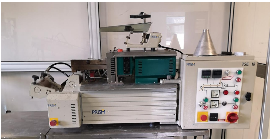
Figure 2-8: Bench-top Prism twin-screw extruder used in this study.
