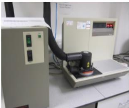
Figure 2-9: TA DSC 2920 used in this study (left-hand side) and schematic diagram of DSC (right-hand side).
