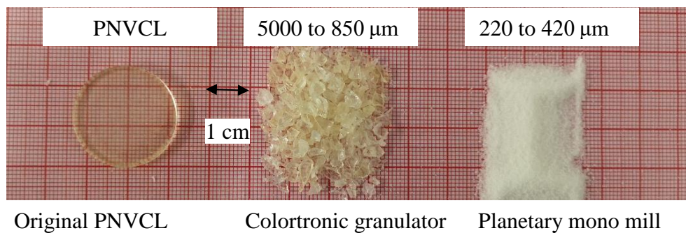
Figure 3-46: A summary of the particle size of PNVCL from photopolymerisation to granulates and powder.
