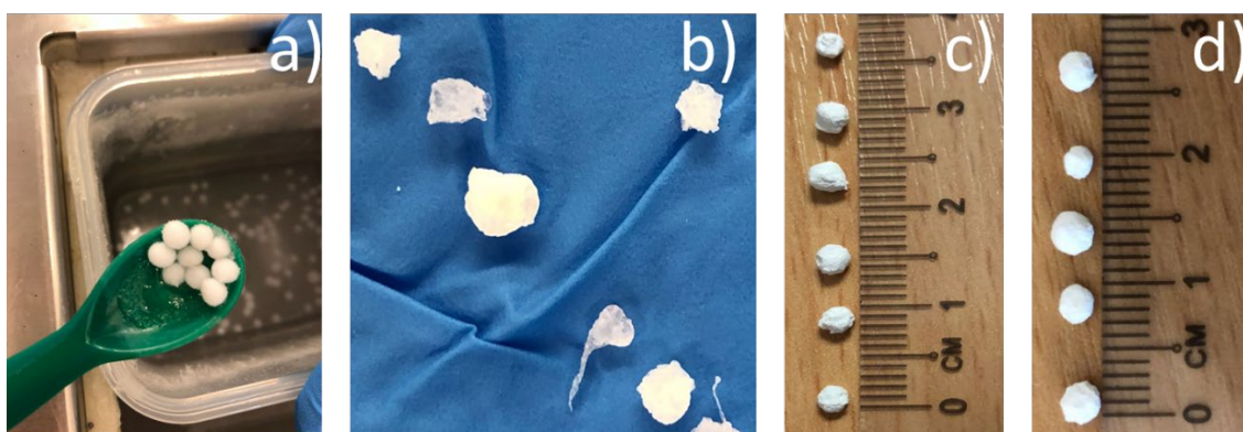
Figure 4.1: (a) Spheres frozen by the dipping method; (b) Samples after freeze-thawing and following freeze-drying; (c) Samples after freezing cycles and (d) Samples after freezing cycles and thawing following freeze-drying.
