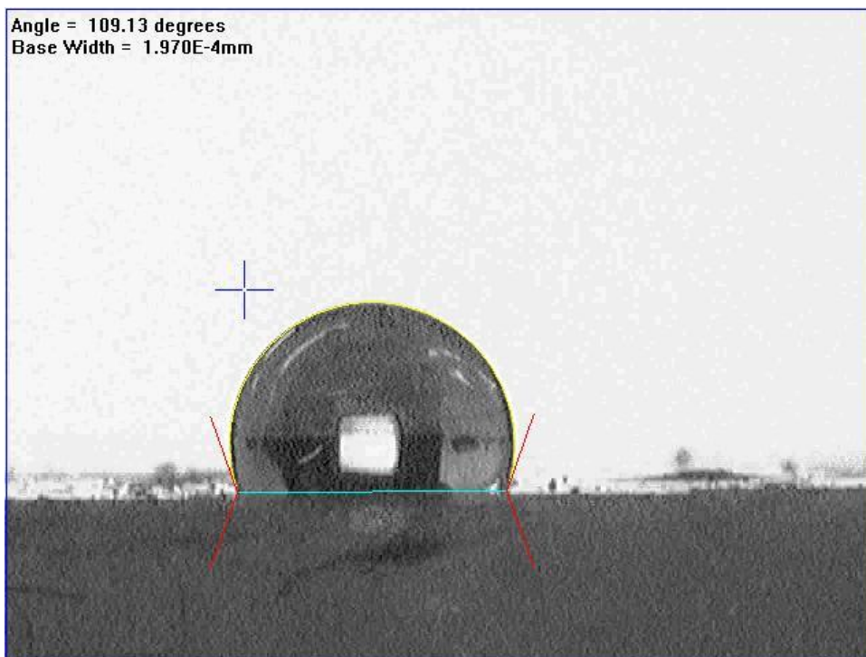
Figure E.4 Sample water droplet from Goniometry measurement, taken for unhydrated PEGDMA-DiPETMP sample (image taken at time 0)
