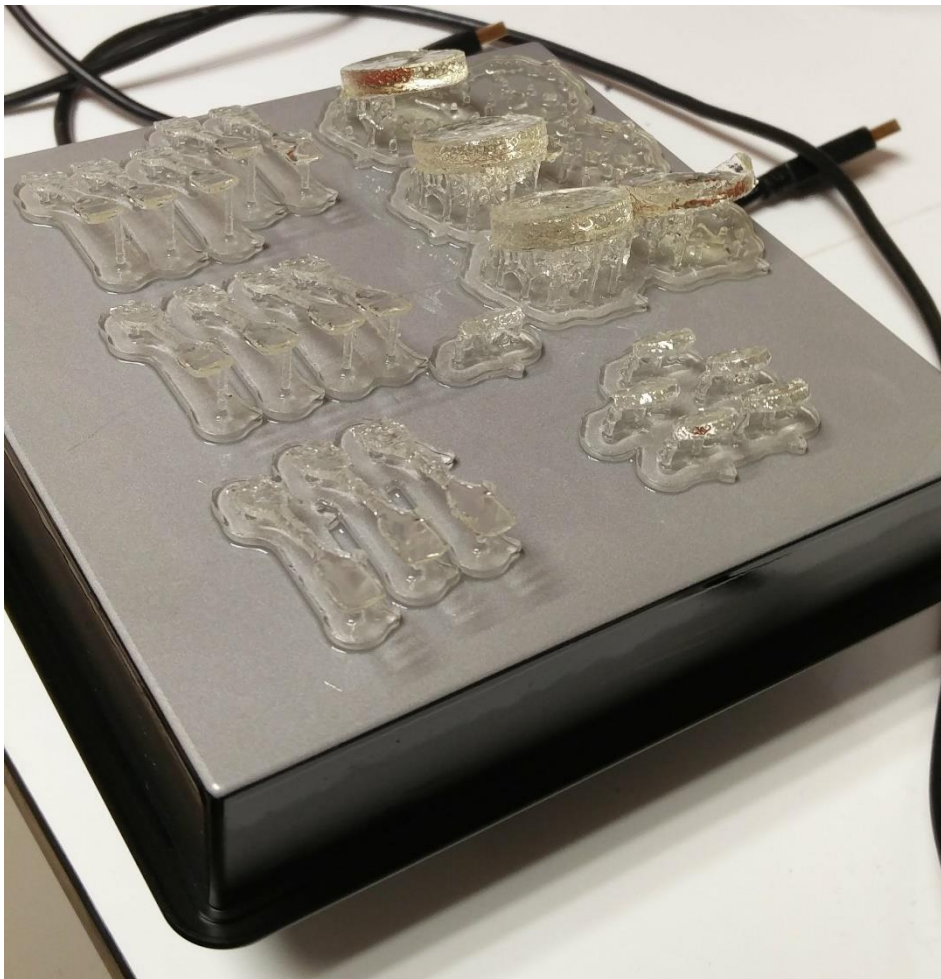
Figure H.1 Printing outcomes for original PEGDMA samples by Stereolithography
