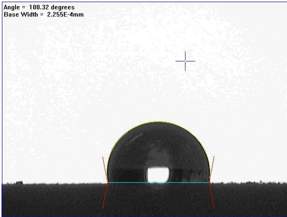
Figure E.5 Sample water droplet from Goniometry measurement, taken for unhydrated Final composition containing PEGDMA, DiPETMP, Bioglass, NAC, Ibu and Prog (image taken at time 0)
