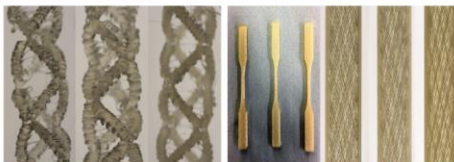
Fig 7. Photographs from optical microscope of 3D printed implants of (a) PLA, (b) PLA/HNT 3% and (c) PLA/HNT 5% nanocomposites. 3D printed tensile bars (a) (L-R) PLA, PLA/HNT 3% and PLA/HNT 5% nanocomposites. (b) Zoomed in photograph of PLA (c) zoomed in photograph of PLA/HNT 3% and (d) zoomed in photograph of PLA/HNT 5% nanocomposite indicates the infill pattern becomes denser with increase in the nanoclay percentage along with change in colour.
