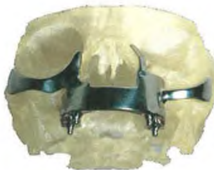
Figure 2.12 Customised maxillofacial implant designed on biomodel [35]
