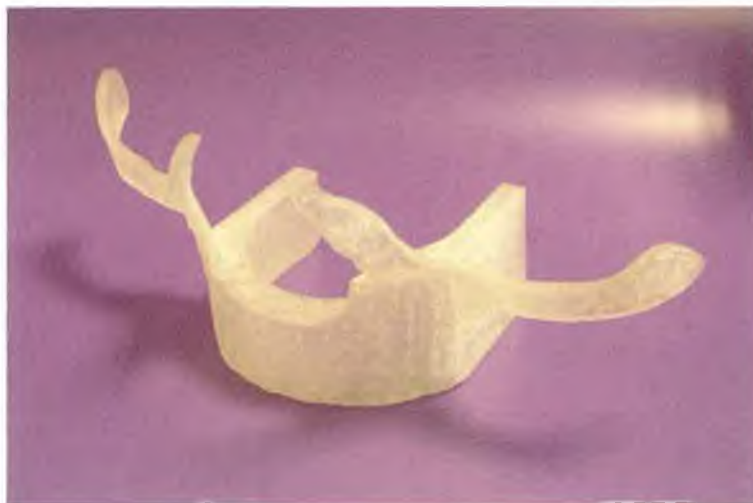
Figure 3.18 SLA RP model used as mould for casting
