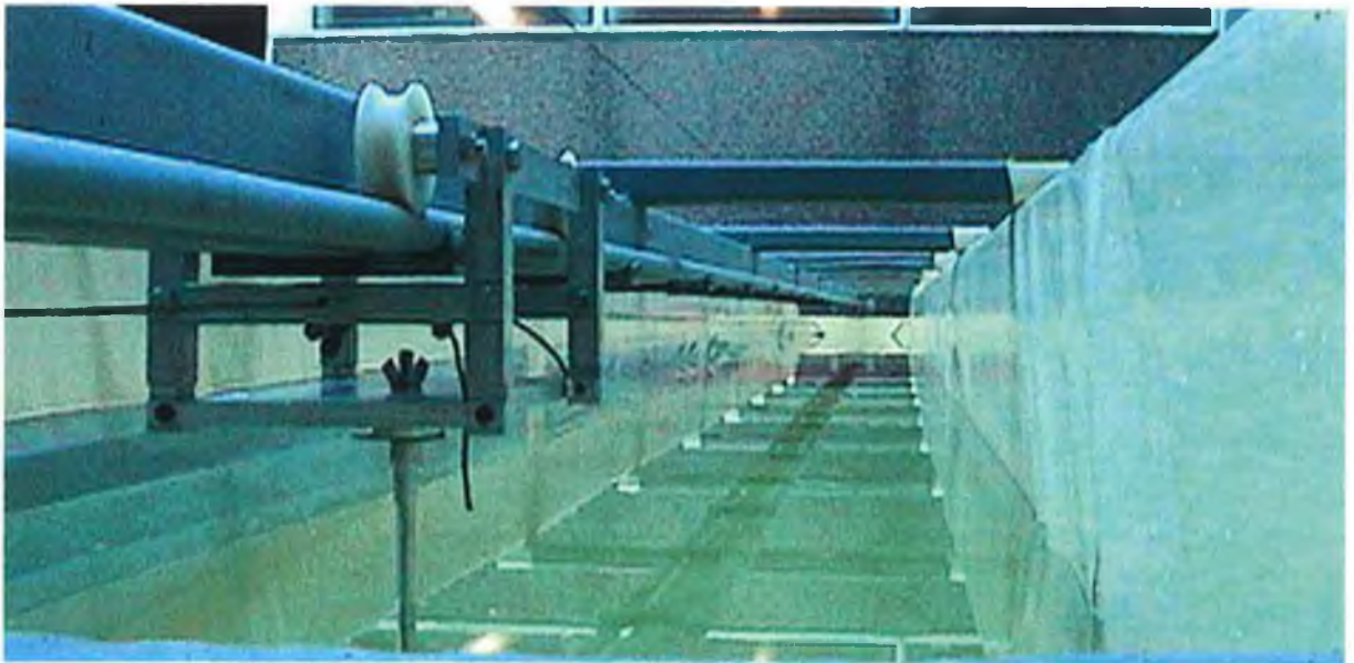
Figure 75 Inside view of the towing tank partially on water, including the rail and the trolley:
