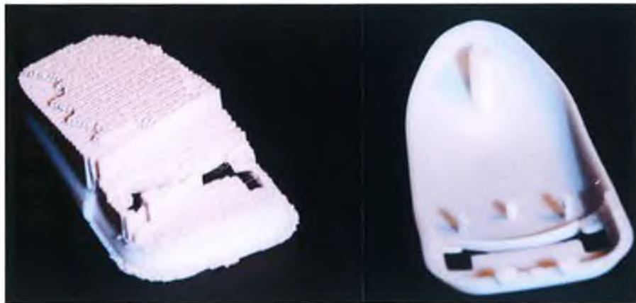
Figure 8.9: FDM Model with supports (before post-processing)
