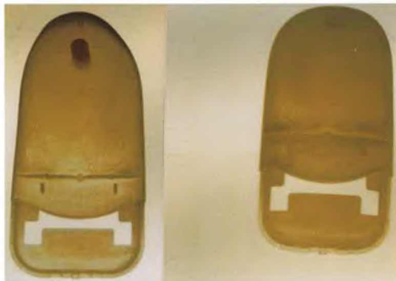
Figure 8.9: FDM Model with supports (before post-processing)
