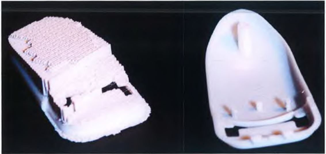
FDM Computer Mouse Top with Build Supports
