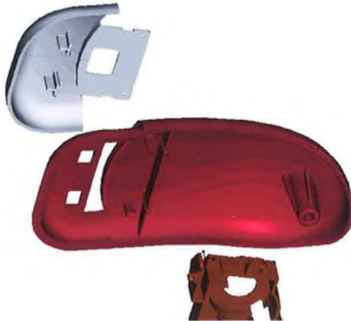
Figure 3.10: Solid Components and Additional Features
