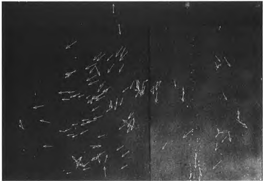
Figure 5-14: shot of the flow beside the cargo with the velocity vectors plotted in.
