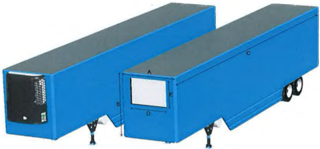
Figure 3-3: General dimensions of a refrigerated trailer
