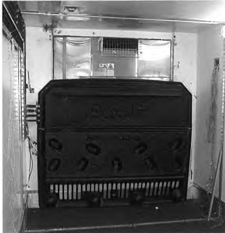
Figure 2-27: A bulkhead fitted in a refrigerated unit
