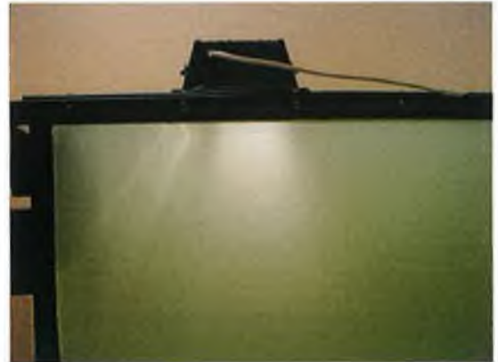
Figure 4-7: Metal-Halide lamp illuminating the particles in the tank
