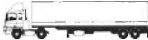
Figure 2-1: Truck with the cargo space on a separate trailer chassis
