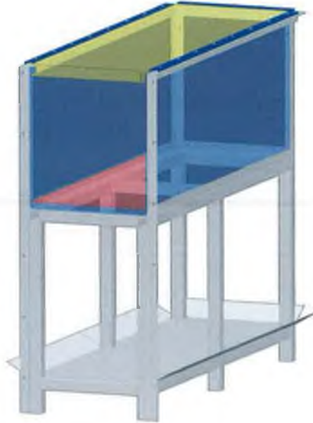
Figure 3-5: The use of a false floor solves the problem of the lost view
