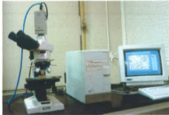
Fig.5.18 Stereomicroscope equipped with a digital camera linked to a computer.
