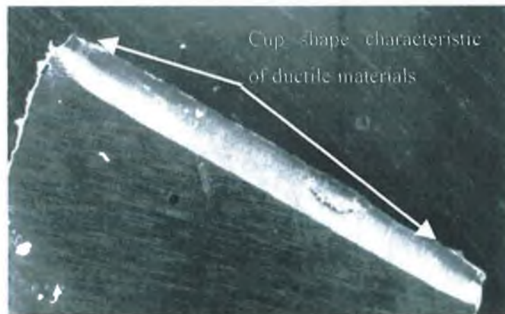
Fig.5.15 X2500 SEM picture showing the cup shape characteristic of ductile fracture.
