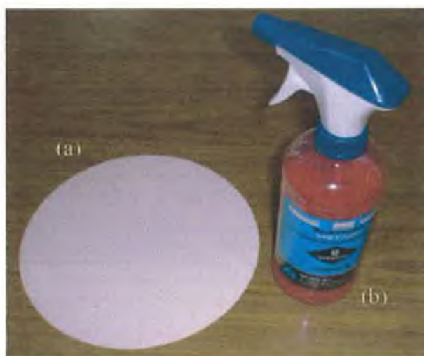
Fig.II.8 (a) Ultrapad, (b) Metadi Diamond Suspension 9 \mu\text{m} .
