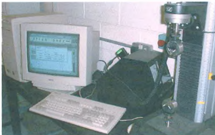
Fig.3.2 Computer linked to the tensile tester.
