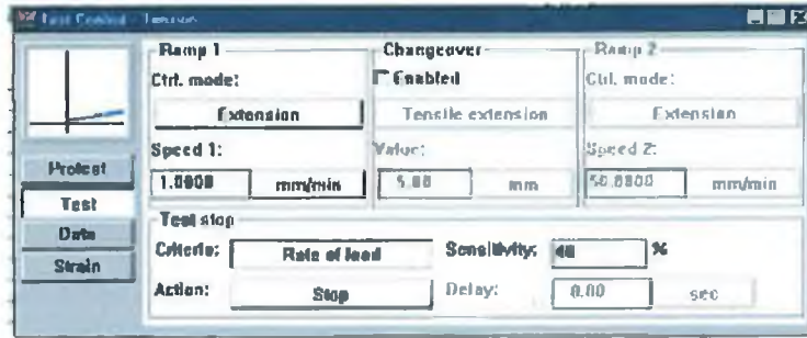
Fig.3.3 Input of the speed and criteria to end the test.
