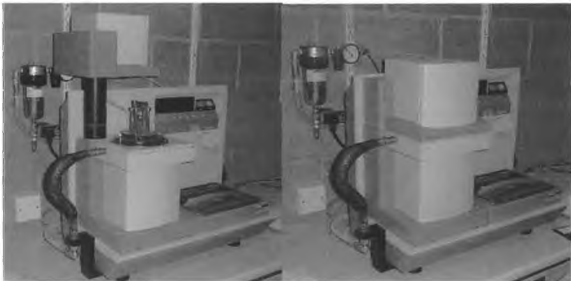
Fig.4.6 Picture of the Dynamic Mechanical Analyser DMA in NCBES, NUIGalway.
