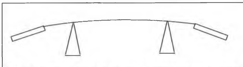
Fig.4.13 Strut bending under the weight of the left over part of tubes.
