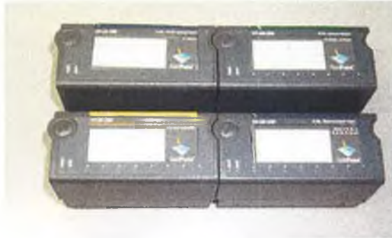
Figure H.5 Field- Point Modules, Ethernet TCP/IP network connection.
