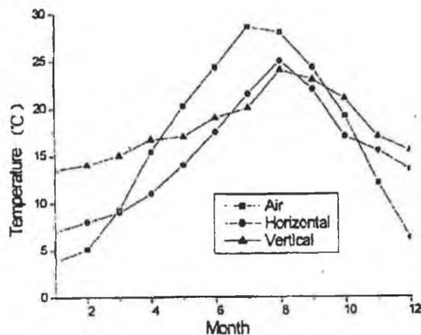
FIGURE 2.5 MONTHLY AVERAGE AIR AND GROUND TEMPERATURES IN HANGZHOU, CHINA (LI *ET AL.*, 2003).
