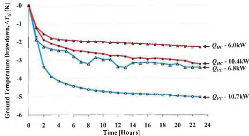
**FIGURE 7.5** COMPARING THE DRAWDOWN OF THE GROUND TEMPERATURE IN THE VICINITY OF BOTH THE HORIZONTAL COLLECTOR ( $\Delta T_{HC,G}$ ) AND THE VERTICAL COLLECTOR ( $\Delta T_{VC,G}$ ) VERSUS EXTRACT RATES ( $Q$ ), RESULTS WERE OBTAINED FROM TESTS CARRIED OUT ON VARIOUS DATES IN 2007.
