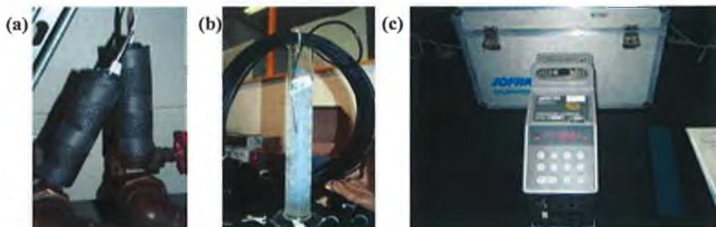
FIGURE F.2 (A) HEAT PUMP COLLECTOR FLOW AND RETURN TEMPERATURE SENSORS IN SITU, (B) TEMPERATURE SENSOR ICE BATH CALIBRATION AND (C) ZOFRA TEMPERATURE SENSOR CALIBRATOR.
