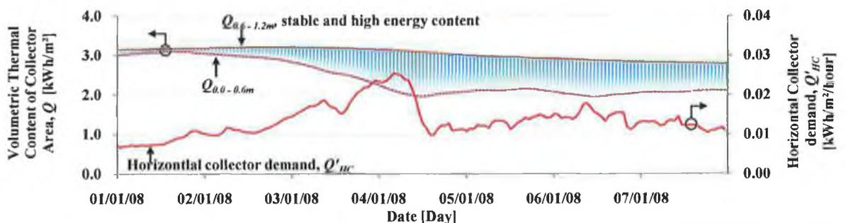
**FIGURE 4.11** THERMAL ENERGY CONTENT WITHIN A 600MM THICK LAYER CENTRED AT DEPTHS OF 0.3M AND 0.9M IN PROFILE 1 VERSUS A PROJECTED COLLECTOR THERMAL DEMAND AT PEAK HEATING SEASON, JANUARY, 2008.
