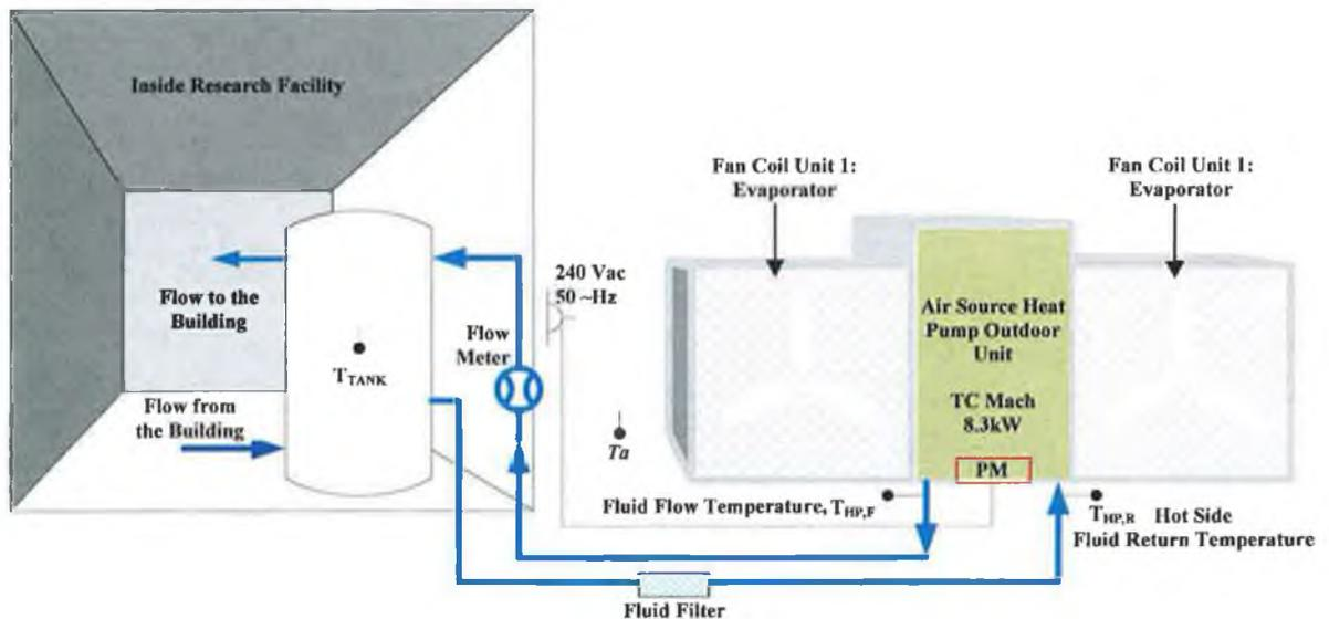
**FIGURE 3.26** CONFIGURATION OF THE ASHP AND MEASUREMENT INSTRUMENTATION.
