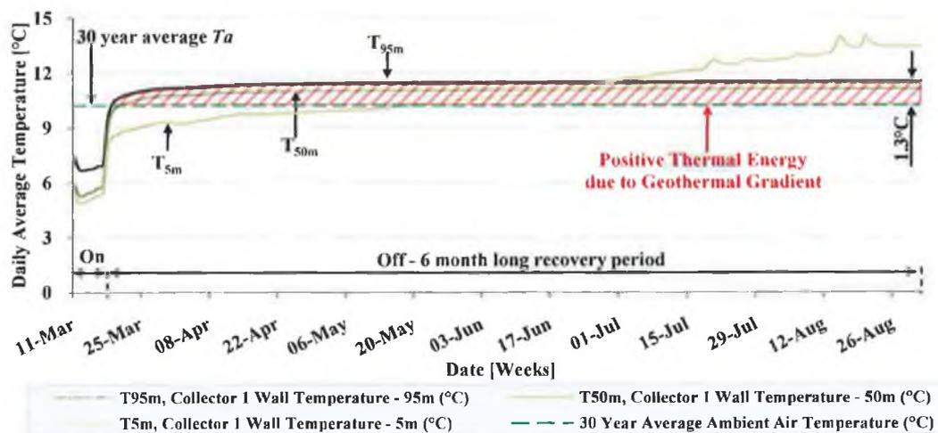
FIGURE 6.3 GEOTHERMAL GRADIENTS ALONG THE HP-IRL VERTICAL COLLECTOR DURING THE RECOVERY PERIOD FOLLOWING TEST VC1 (MARCH-AUGUST 2007).
