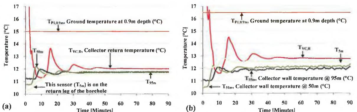
FIGURE 6.5 *HP-IRL* VERTICAL COLLECTOR (BOREHOLE 1) FARFIELD GROUND TEMPERATURE IN (A) MAY 2008 AND (B) JULY 2009.
