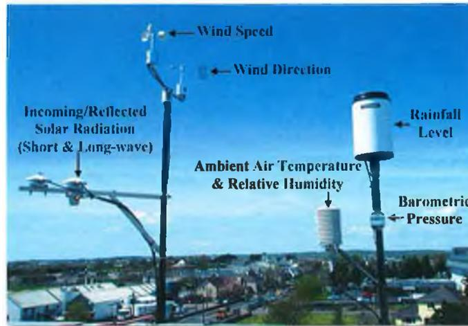
FIGURE 3.9 IBC’S ROOF MOUNTED, AUTOMATED WEATHER STATION INSTALLED IN 2006.
