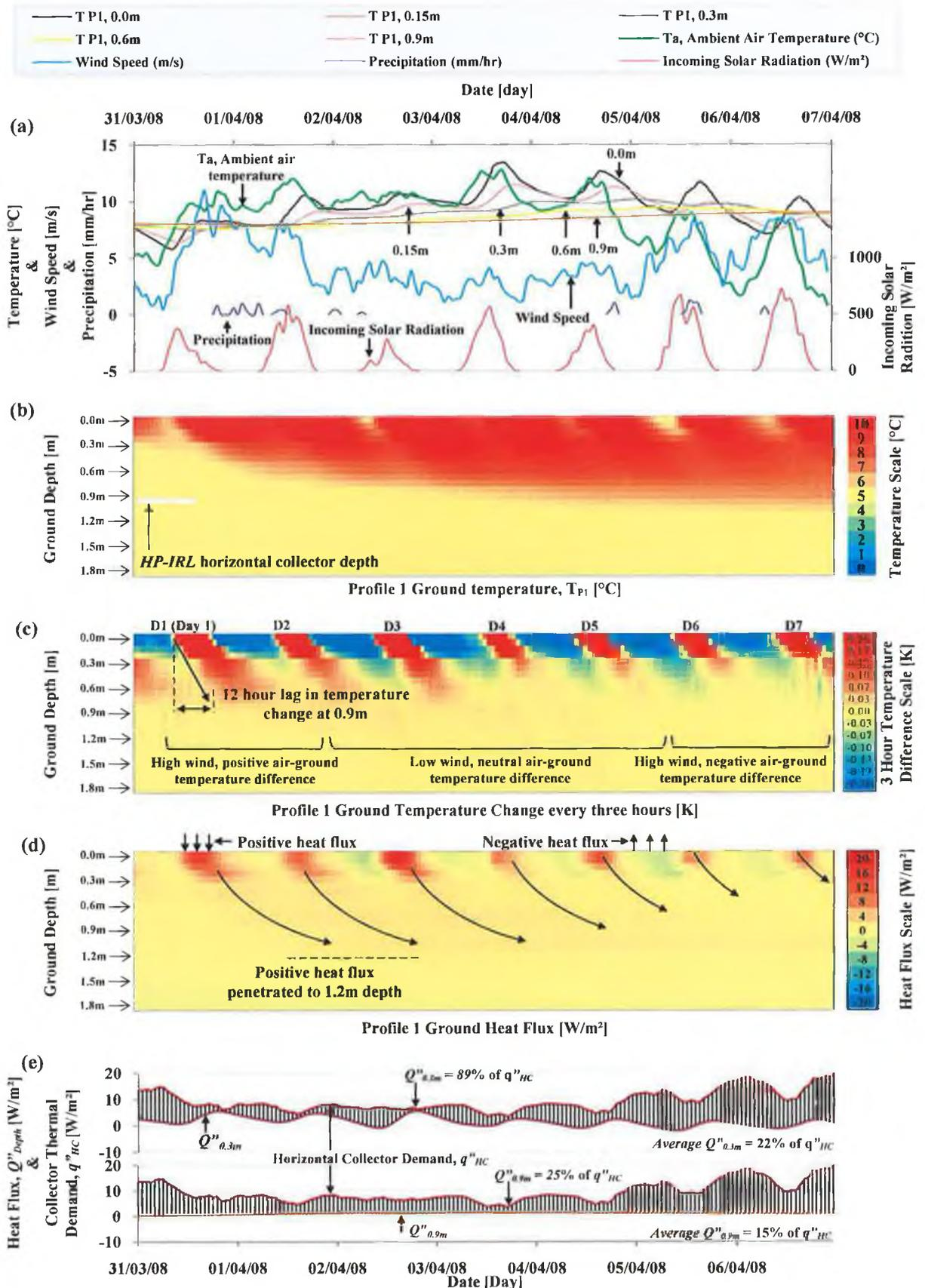
**FIGURE 4.12** FIRST WEEK IN APRIL, 2008, HOURLY AVERAGED (A) WEATHER PARAMETERS AND PROFILE 1 GROUND TEMPERATURE, (B) 3-D TRANSIENT TEMPERATURE MAP OF PROFILE 1, (C) 3-D TRANSIENT TEMPERATURE CHANGE MAP SHOWING THE RATE OF GROUND TEMPERATURE CHANGE EVERY THREE HOURS AT PROFILE 1, (D) TRANSIENT GROUND HEAT FLUX MAP AND (E) GROUND HEAT FLUX IN COMPARISON TO THEORETICAL HORIZONTAL COLLECTOR THERMAL DEMAND.
