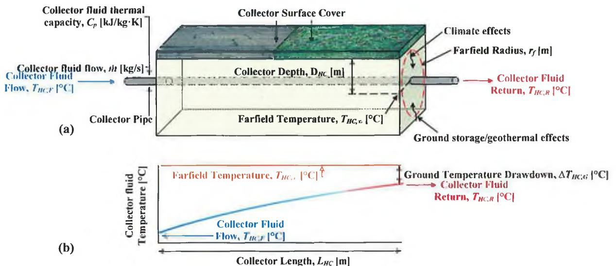
FIGURE 5.1 HORIZONTAL COLLECTOR (A) DESIGN AND PERFORMANCE INDICATORS AND (B) COLLECTOR FLUID TEMPERATURE CHANGE WITH COLLECTOR LENGTH.
