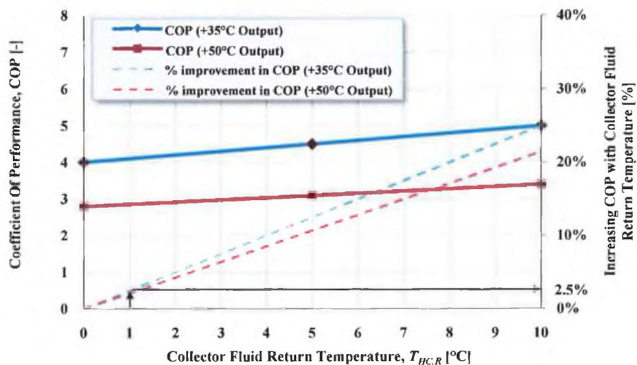
FIGURE 4.18 PERCENTAGE IMPROVEMENT IN *HP-IRL* COP WITH INCREASED COLLECTOR FLUID RETURN TEMPERATURE.
