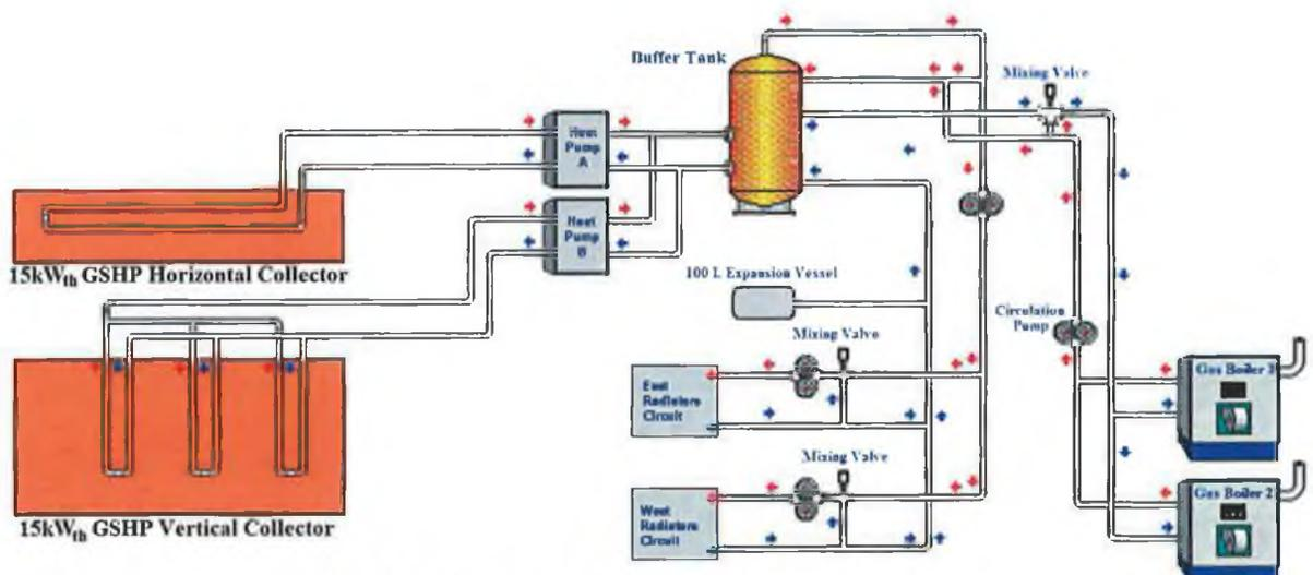
FIGURE 3.3 THE IIBC HEATING SYSTEM SCHEMATIC.
