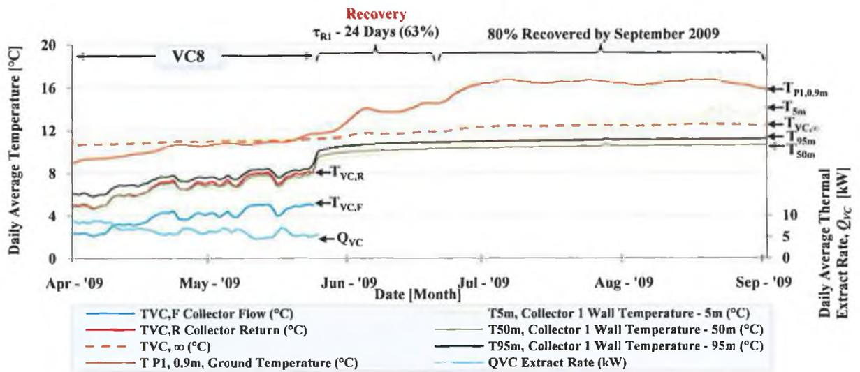
FIGURE 6.15 TEST PERIOD VC8 AND VERTICAL BOREHOLE THERMAL RECOVERY AFTER THREE CONSECUTIVE YEARS OPERATION.
