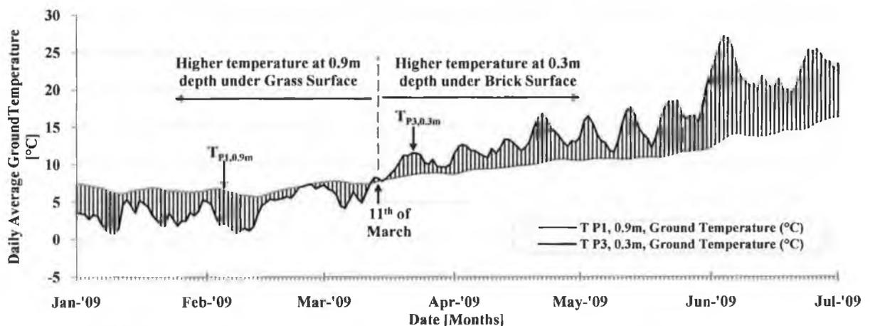
FIGURE 4.41 WINTER, SPRING AND SUMMER GROUND TEMPERATURE DIFFERENCES UNDER GRASS SURFACE (0.9M) AND UNDER BRICK PAVEMENT SURFACE (0.3M).
