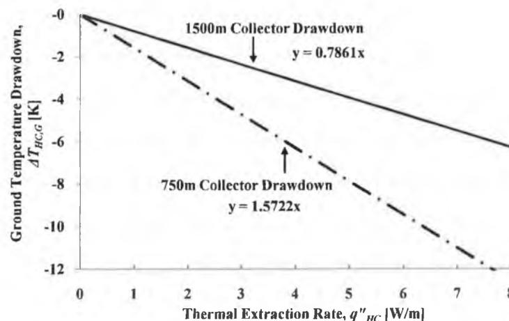
**FIGURE 5.8** PREDICTED GROUND TEMPERATURE DRAWDOWN WITH THERMAL EXTRACTION RATE PER M OF COLLECTOR PIPE FOR 750M AND 1500M COLLECTORS WITH 0.3M PIPE SPACING.
