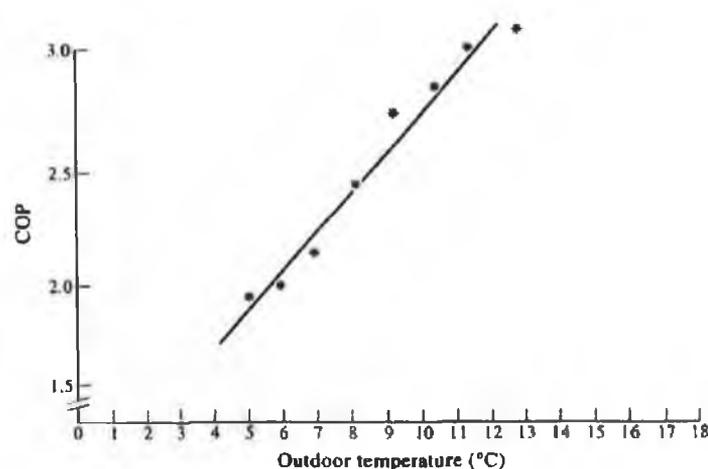
**FIGURE 2.14** VARIATION IN ASHP COP WITH AMBIENT AIR TEMPERATURE (KENT, 1997).
