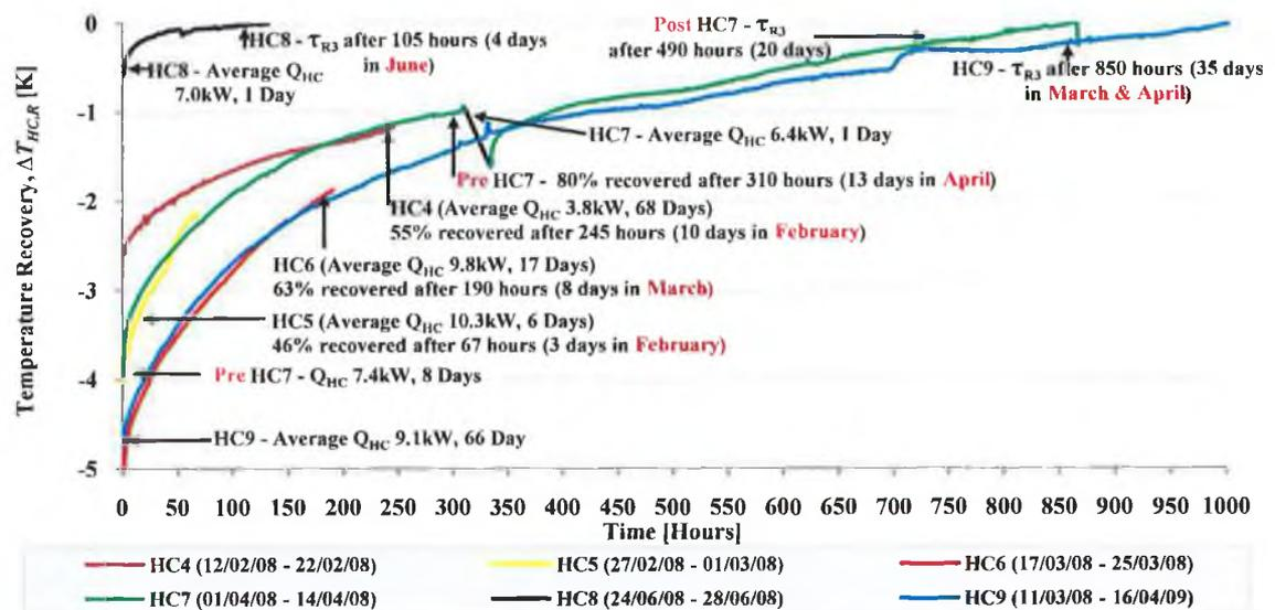
FIGURE 4.24 THERMAL RECOVERY OF THE COLLECTOR REGION WITHIN PROFILE 5 AFTER TEST PERIODS HC4 THROUGH HC9.
