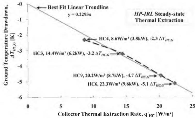
**FIGURE 4.23** GROUND TEMPERATURE DRAWDOWN ( $\Delta T_{HC,G}$ ) RECORDED UNDER STEADY-STATE THERMAL EXTRACTION CONDITIONS DURING TEST PERIODS HC3, HC4, HC6 AND HC9.
