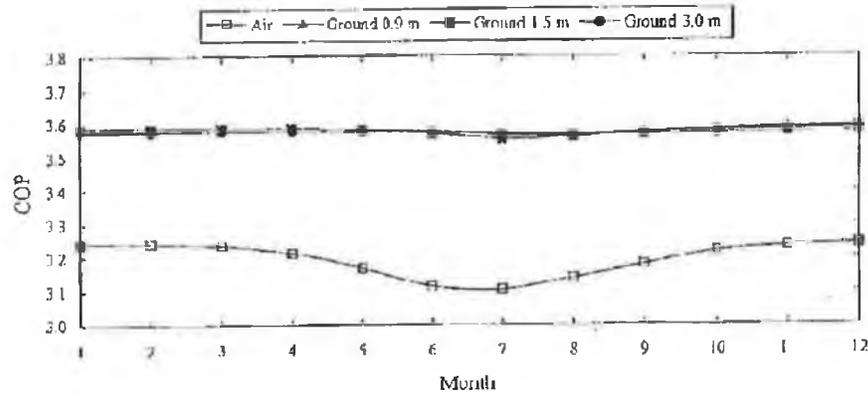
**FIGURE 2.16** PREDICTED MONTHLY HEATING COPs FOR AIR AND GROUND SOURCE HEAT PUMP SYSTEMS (DE SWARDT AND MEYER, 2001).
