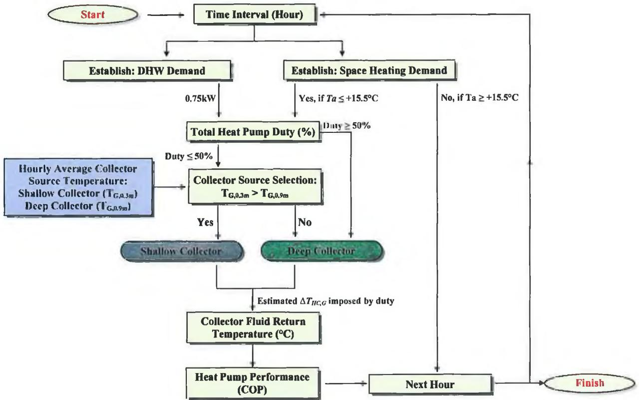
FIGURE 5.10 SPLIT LEVEL HORIZONTAL COLLECTOR GSHP SIMULATION DECISION TREE BASED ON THREE YEARS OF HOURLY AVERAGED TEMPERATURE DATA (2007-2009).
