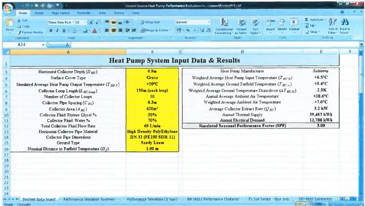
FIGURE L.1 SCREEN-GRAB OF GSHP PERFORMANCE EVALUATION TOOL USING THREE YEARS OF MARITIME CLIMATE DATA AND SOLTERRA HEAT PUMP PERFORMANCE CHARACTERISTICS, AS PER TEST STANDARD EN 14511.
