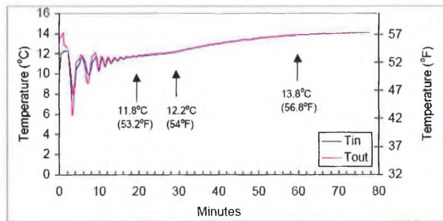
FIGURE 6.4 VERTICAL COLLECTOR FARFIELD GROUND TEMPERATURE IN LULEÅ SWEDEN (GEHLIN, 2002).
