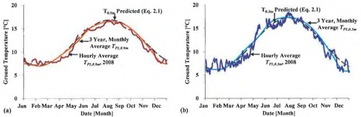
**FIGURE 4.3** COMPARISON OF *HP-IRL* MEASURED HOURLY AND MONTHLY AVERAGED GROUND TEMPERATURE OF PROFILE 1 AT (A) 0.9M DEPTH BETWEEN 2007 AND 2009 WITH THAT OF THE PREDICTED GROUND TEMPERATURES AT 0.9M AND (B) 0.3M DEPTH BETWEEN 2007 AND 2009 WITH THAT OF THE PREDICTED GROUND TEMPERATURES AT 0.3M.
