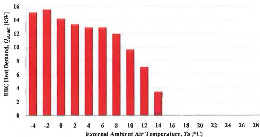
**FIGURE 3.5** TOTAL HEAT DEMAND OF THE IiBC FROM THE HEAT PUMPS AS A FUNCTION OF EXTERNAL AMBIENT AIR REQUIREMENTS.
