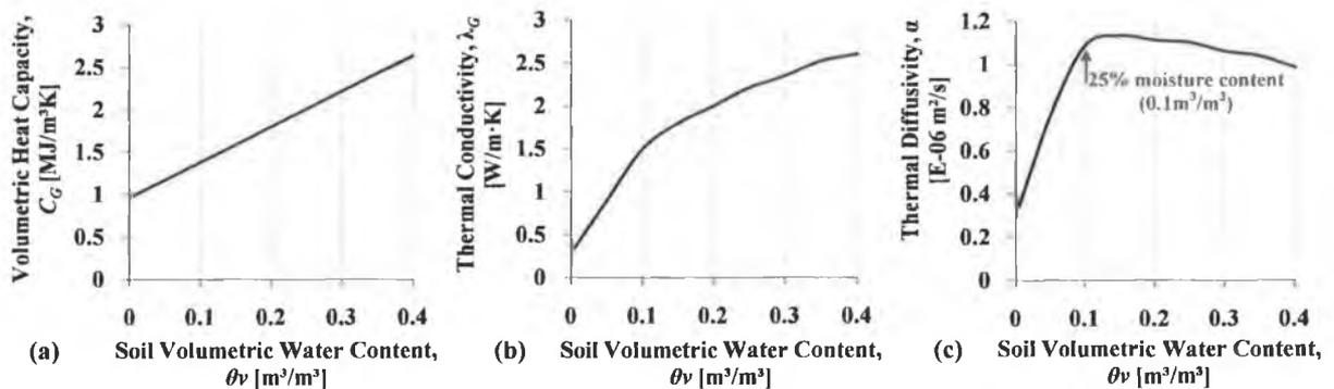
**FIGURE 2.8** (A) VARIATION IN VOLUMETRIC HEAT CAPACITY WITH MOISTURE CONTENT FOR IRISH SANDY/SILTY LOAM SOIL WITH AN AVERAGE BULK DENSITY OF  $1200\text{KG}/\text{M}^3$  (B) VARIATION OF SOIL THERMAL CONDUCTIVITY, AND (C) VARIATION OF THERMAL DIFFUSIVITY (WITH INCREASED IN SOIL MOISTURE CONTENT FOR IRISH SANDY LOAM SOIL WITH AN AVERAGE BULK DENSITY OF  $1200\text{KG}/\text{M}^3$ ) (LOHAN *ET AL.*, 2006).
