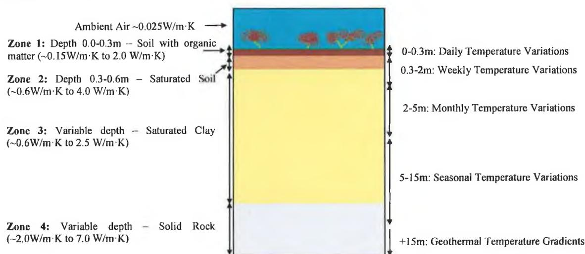
FIGURE 2.7 GROUND TEMPERATURE AND CONDUCTIVITY VARIATIONS WITH DEPTH.
