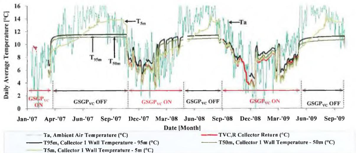
**FIGURE 6.2** VERTICAL COLLECTOR (BOREHOLE 1) WALL TEMPERATURES AT 5M, 50M AND 95M BETWEEN 2007 AND 2009.
