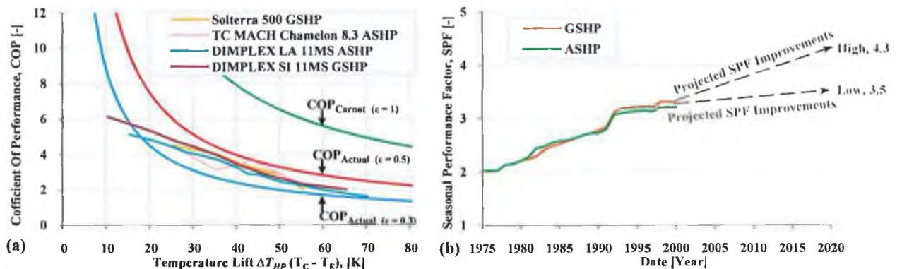
**FIGURE 1.3** (A) MANUFACTURER DEFINED EXAMPLES OF HEAT PUMP COP VERSUS TEMPERATURE LIFT FOR GSHP AND ASHPs AND (B) SPF IMPROVEMENTS OVER PAST 25 YEARS (LAZZARIN, 2007), WITH POTENTIAL FUTURE IMPROVEMENT TRENDS.
