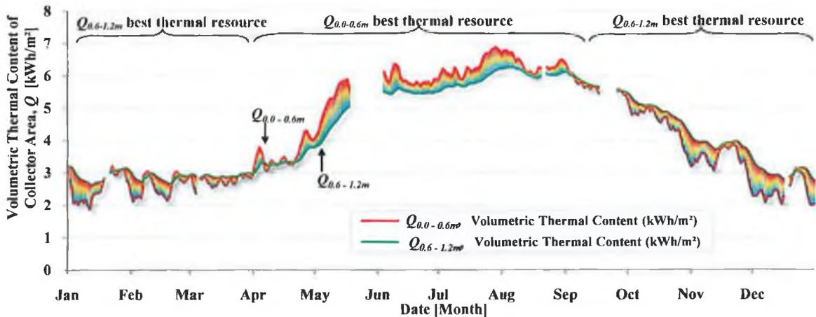
FIGURE 4.14 THERMAL ENERGY CONTENT OF GROUND AT 0.3M AND 0.9M DEPTHS FOR 2008.
