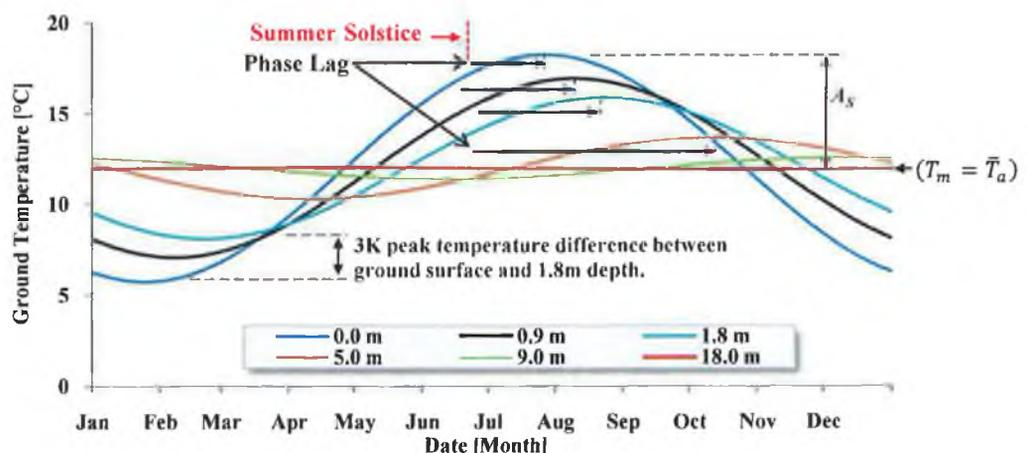
FIGURE 2.9 PREDICTED GROUND TEMPERATURE VARIATIONS WITH DEPTH FOR THE GROUND CONDITIONS IN THE HP-IRL STUDY.
