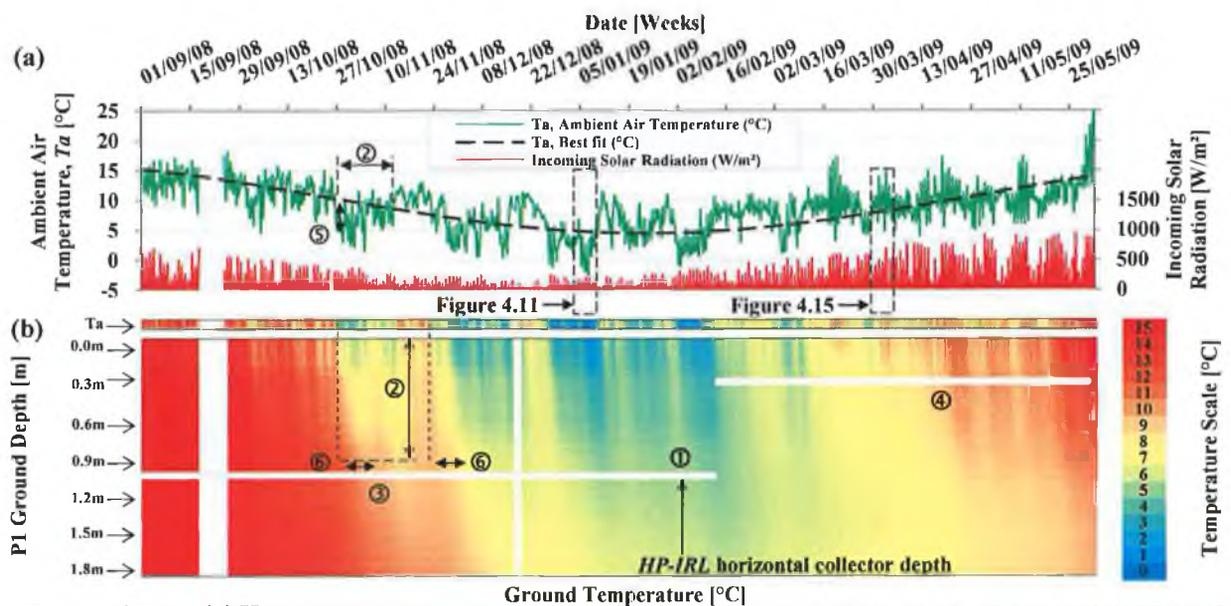
**FIGURE 4.7** (A) HOURLY AVERAGED AMBIENT AIR TEMPERATURE AND INCOMING SOLAR RADIATION DRIVING (B) 3-D TRANSIENT TEMPERATURE MAP OF THE GROUND THERMAL CHARGE AND DISCHARGE AT PROFILE 1 DURING HEATING SEASON FROM SEPTEMBER 2008 TO MAY 2009.
