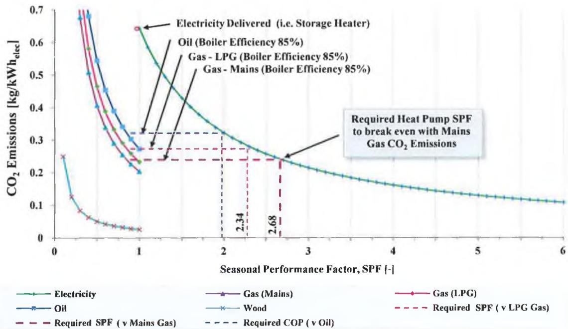
**FIGURE 7.9** CO<sub>2</sub> EMISSIONS FROM VARIOUS HEATING SYSTEMS AS A FUNCTION OF HEAT PUMP SPF.
