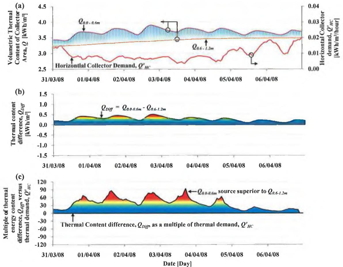
**FIGURE 4.13** (A) AVAILABLE THERMAL ENERGY AT 0.3M AND 0.9M DEPTHS VERSUS THEORETICAL COLLECTOR THERMAL DEMAND, (B) VOLUMETRIC THERMAL ENERGY DIFFERENCE BETWEEN  $Q_{0.0-0.6m}$  AND  $Q_{0.6-1.2m}$  AND (C) VOLUMETRIC THERMAL ENERGY DIFFERENCE BETWEEN  $Q_{0.0-0.6m}$  AND  $Q_{0.6-1.2m}$  AS A MULTIPLE OF HORIZONTAL COLLECTOR THERMAL DEMAND,  $Q'_{HC}$ .
