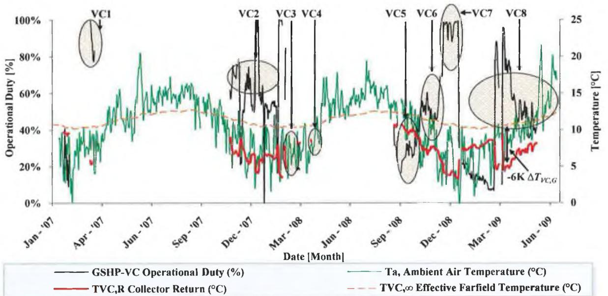
FIGURE 6.7 TIMING OF THE EIGHT GSHP<sub>VC</sub> TEST PERIODS (2007-2009) AND CORRESPONDING DUTY.
