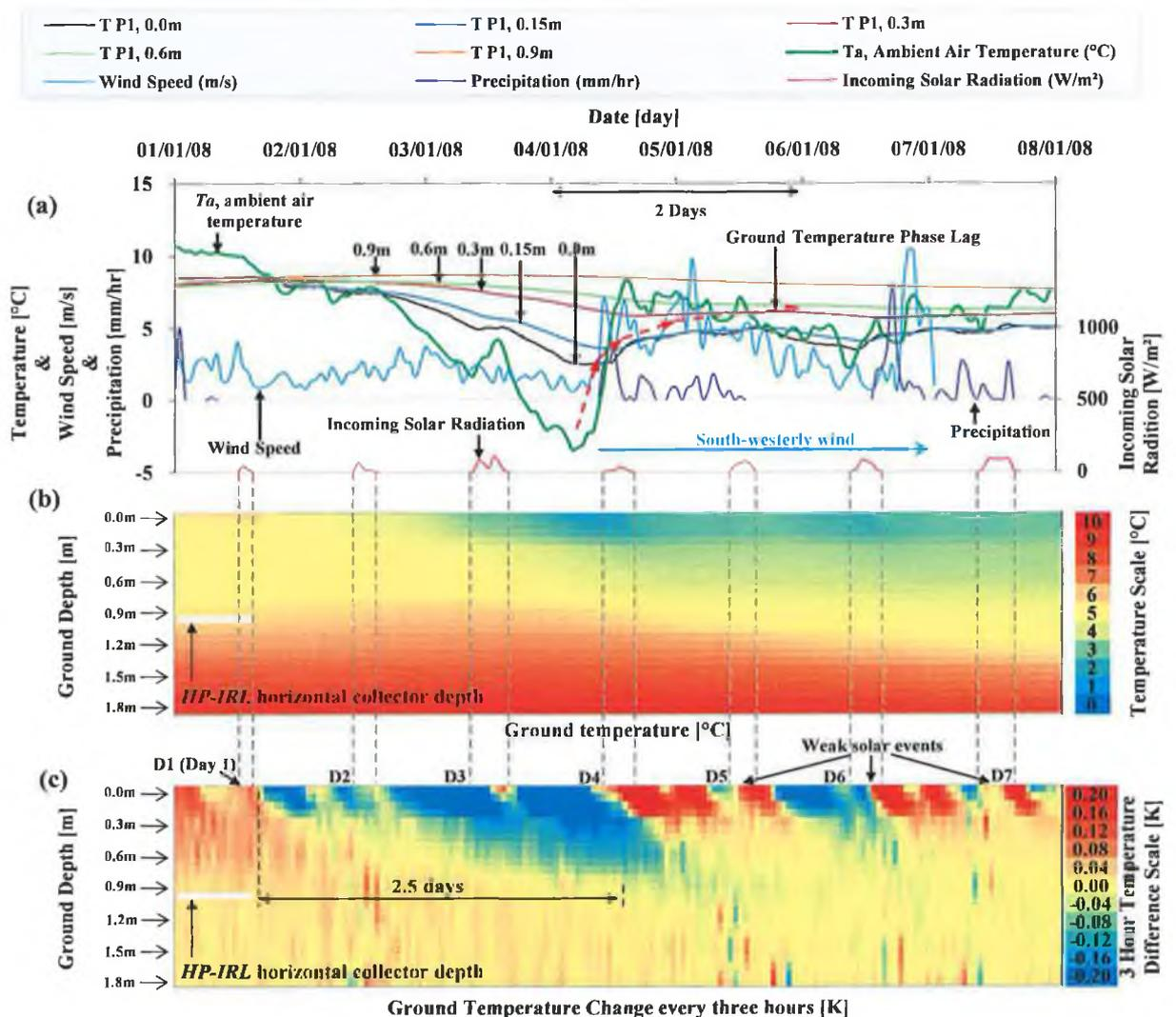
**FIGURE 4.10** FIRST WEEK IN JANUARY, 2008, HOURLY AVERAGE (A) TRANSIENT WEATHER PARAMETERS AND PROFILE 1 GROUND TEMPERATURE, (B) 3-D TRANSIENT TEMPERATURE MAP AT PROFILE 1 AND (C) 3-D TRANSIENT TEMPERATURE CHANGE MAP OF THE RATE OF GROUND TEMPERATURE CHANGE EVERY THREE HOURS.
