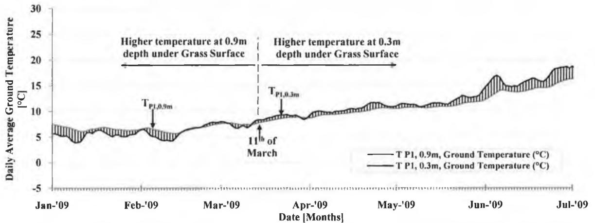
FIGURE 4.40 WINTER, SPRING AND SUMMER GROUND TEMPERATURE DIFFERENCES UNDER GRASS SURFACE AT 0.3M AND 0.9M DEPTH.
