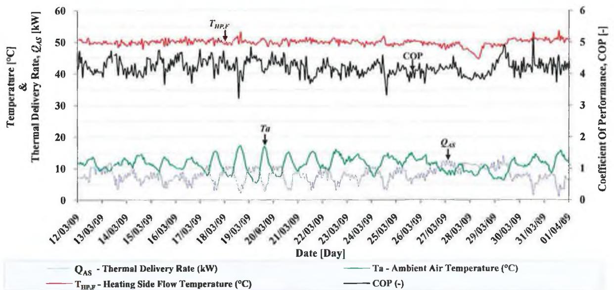
FIGURE 6.25 HOURLY AVERAGED ASHP PERFORMANCE CHARACTERISTICS DURING TEST PERIOD AS4.
