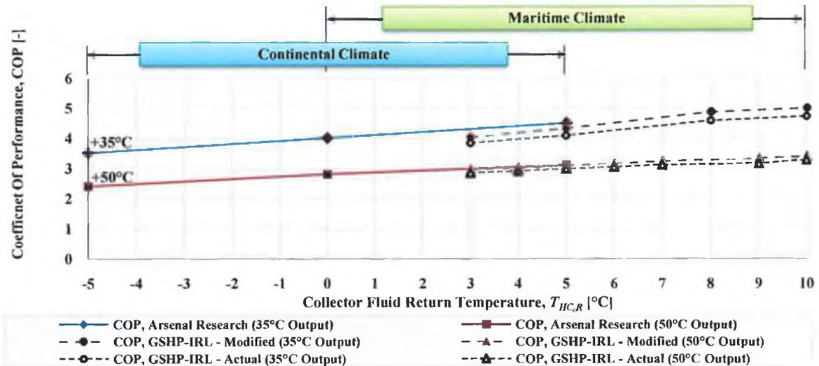
**FIGURE 4.17** COMPARISON OF HEAT PUMP PERFORMANCE AS MEASURED USING INTERNATIONAL STANDARD EN-14511 AND DATA FROM *HP-IRL* STUDY.
