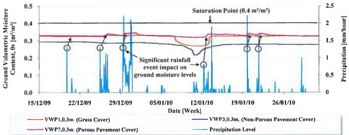
**FIGURE 4.9** RECORDED RAINFALL AND HOURLY AVERAGE GROUND VOLUMETRIC MOISTURE CONTENT IN COLLECTOR REGION AT 0.3M DEPTH (DECEMBER 2009 TO JANUARY 2010).
