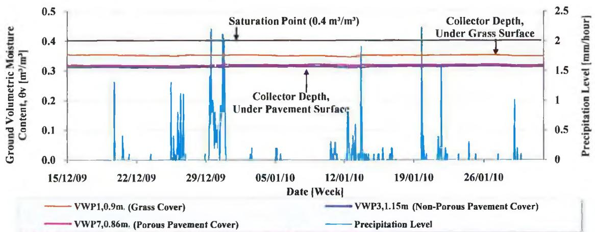
**FIGURE 4.8** RECORDED RAINFALL AND HOURLY AVERAGED GROUND VOLUMETRIC MOISTURE CONTENT AT COLLECTOR DEPTH (DECEMBER 2009 TO JANUARY 2010).
