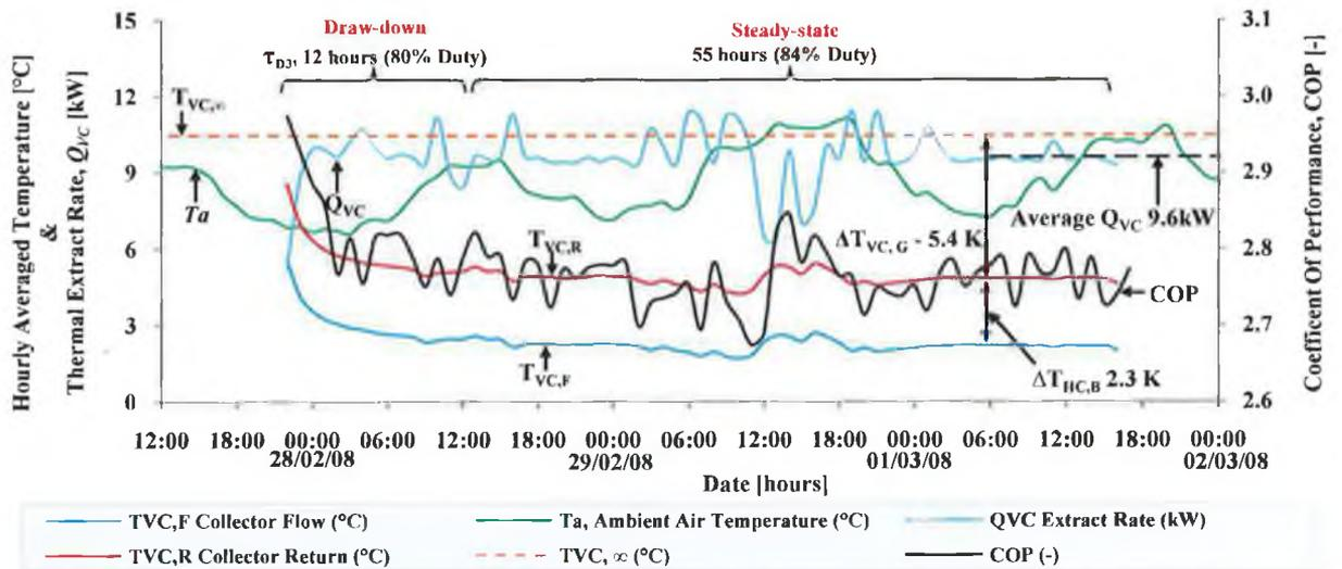
**FIGURE 6.10** HOURLY AVERAGED THERMAL DRAWDOWN AND STEADY-STATE PERFORMANCE DURING TEST PERIOD VC3.
