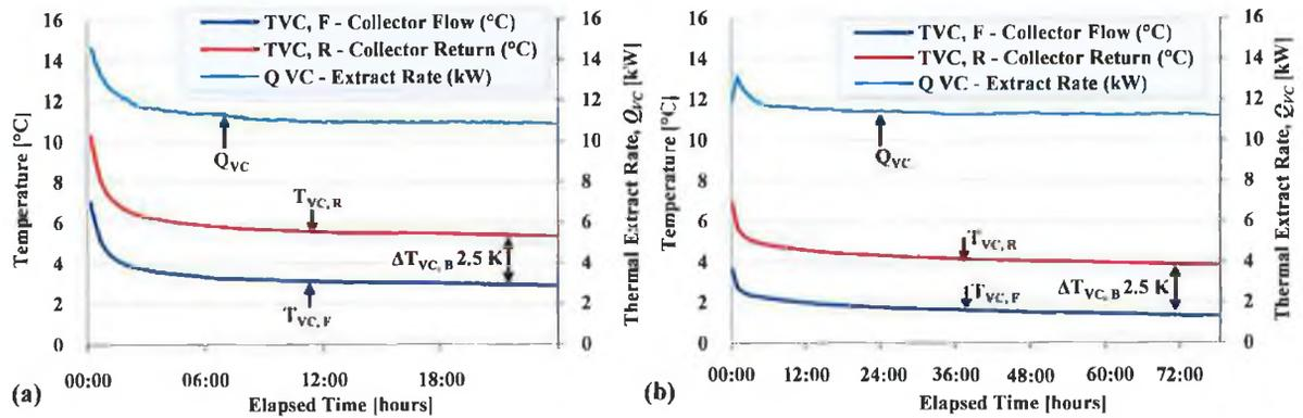
**FIGURE 6.18** MEASURED THERMAL EXTRACTION IN TEST PERIODS (A) OVER ONE DAY, VC1 (11/03/07) AND (B) OVER THREE DAYS, VC2(J) (15/02/08 – 18/02/08) AND ITS IMPACT ON THE COLLECTOR FLUID TEMPERATURES.
