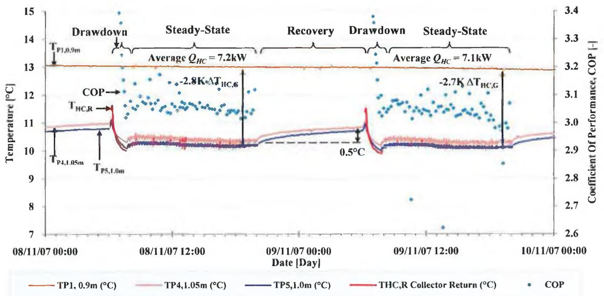
**FIGURE 4.34** DRAWDOWN AND RECOVERY OF THE GROUND TEMPERATURE IN THE GSHP<sub>HC</sub> COLLECTOR REGION DURING NOVEMBER, 2007 (HC3).
