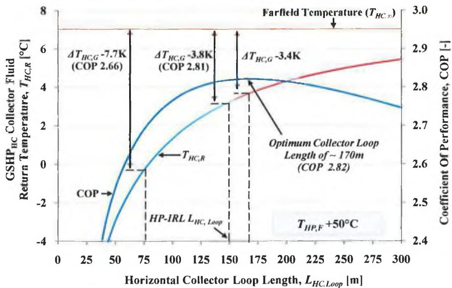
**FIGURE 5.3** VARIATION IN THE COLLECTOR FLUID RETURN TEMPERATURE AND RESULTING COP WITH COLLECTOR LENGTH FOR  $+50^\circ\text{C}$  OUTPUT TEMPERATURE.
