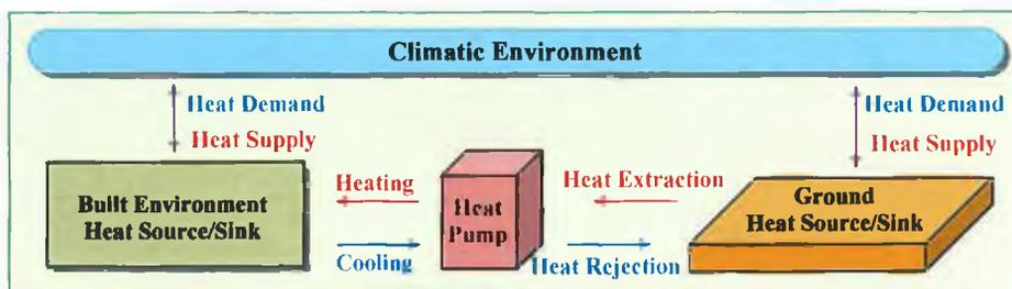
**FIGURE 1.5** INTERDEPENDENCE BETWEEN BUILDING DEMAND, CLIMATE AND HEAT SOURCE/SINK.
