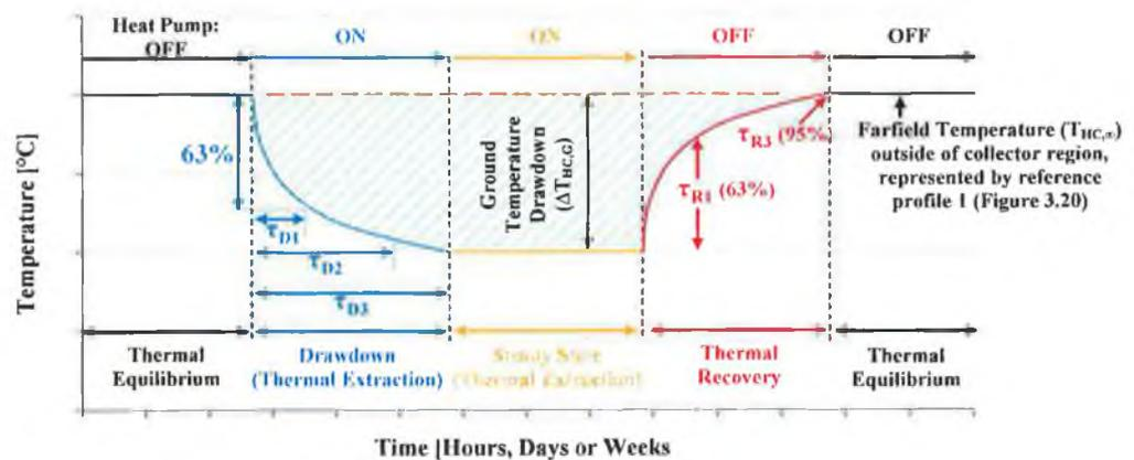
**FIGURE 4.19** SCHEMATIC OF THERMAL EXTRACTION AND RECOVERY CHARACTERISTICS, TO DEFINE DRAWDOWN, STEADY-STATE AND RECOVERY PERIODS ASSOCIATED WITH HEAT PUMP COLLECTOR OPERATION.
