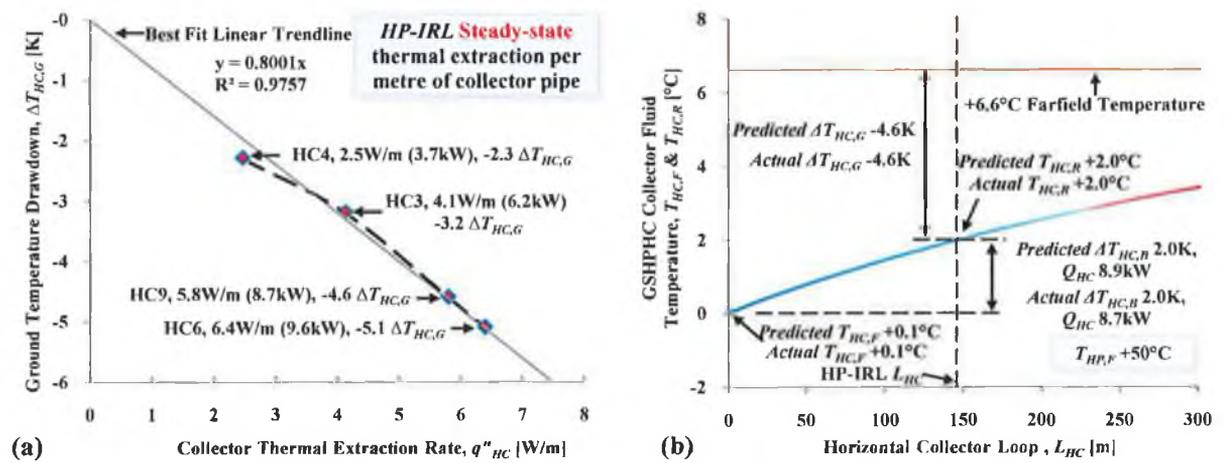
**FIGURE 5.2** (A) GROUND TEMPERATURE DRAWDOWN ( $\Delta T_{HC,G}$ ) VERSUS COLLECTOR THERMAL EXTRACTION RATE PER METER OF COLLECTOR PIPE (1500M) RECORDED UNDER STEADY-STATE THERMAL EXTRACTION CONDITION IN TEST PERIODS HC3, HC4, HC6 AND HC9 AND (B) LONG-TERM STEADY STATE PREDICTED VARIATION TO THE COLLECTOR FLUID TEMPERATURE ALONG THE COLLECTOR LENGTH WHEN EXPOSED TO A UNIFORM FARFIELD GROUND TEMPERATURE OF +6.6°C VERSUS TEMPERATURES RECORDED IN TEST PERIOD HC9.
