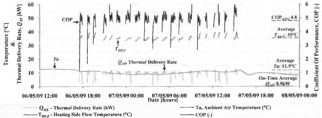
FIGURE 6.26 FIVE MINUTE RECORDING INTERVAL OF THE ASHP PERFORMANCE CHARACTERISTICS DURING TEST PERIOD AS5 WITH +35°C HEAT PUMP FLOW TEMPERATURE ( $T_{HP,F}$ ).
