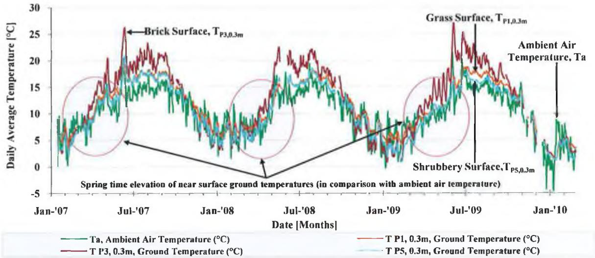
FIGURE 4.38 GROUND TEMPERATURES AT 0.3M UNDER GRASS, BRICK AND SHRUBBERY SURFACES.
