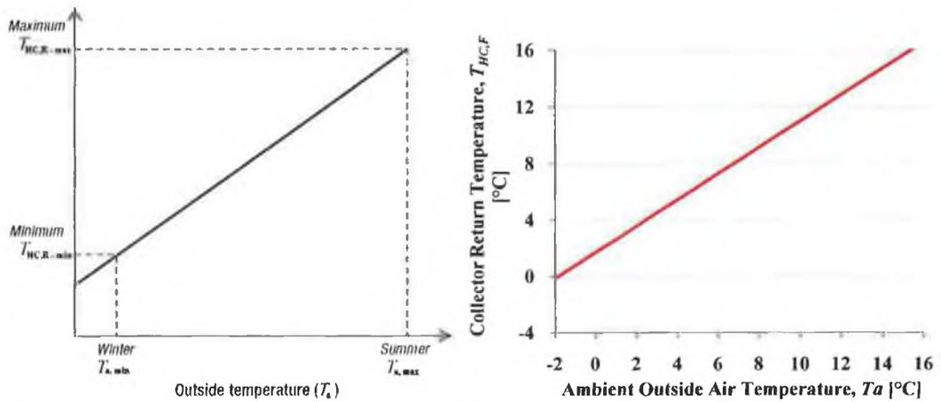
**FIGURE 7.3** ENTERING WATER TEMPERATURE AS (A) A FUNCTION OF EXTERNAL AIR TEMPERATURE (RETSREEN, 2005) AND (B) ENTERING WATER TEMPERATURE AS A FUNCTION OF EXTERNAL AIR TEMPERATURE FOR IRISH CLIMATIC CONDITIONS.
