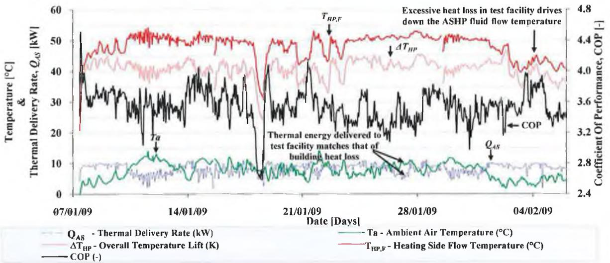
FIGURE 6.23 HOURLY AVERAGED ASHP PERFORMANCE CHARACTERISTICS DURING TEST PERIOD AS2.
