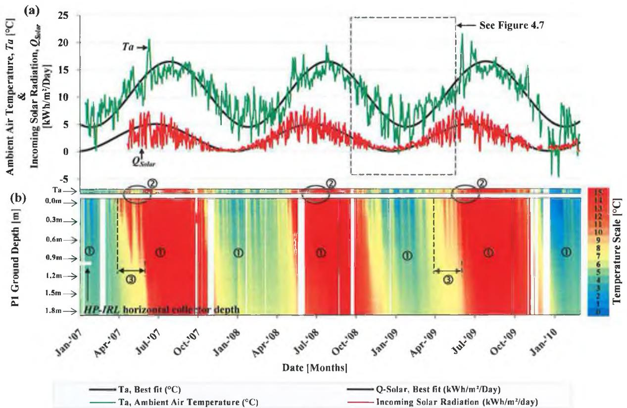
**FIGURE 4.6** (A) DAILY AMBIENT AIR TEMPERATURE AND INCOMING SOLAR RADIATION DRIVING THE THERMAL CHARGE AND DISCHARGE OF THE GROUND IN PROFILE 1 (B) PROFILE 1 3-D TRANSIENT TEMPERATURE MAP SHOWING HOURLY GROUND TEMPERATURE VARIATION WITH DEPTH TO 1.8M.
