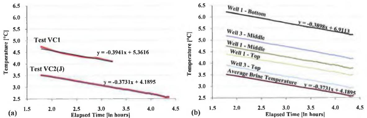
**FIGURE 6.19** NATURAL LOG PROGRESSION OF THERMAL EXTRACTION FOR (A) TWO TIME PERIODS VC1 AND VC2(J) AND (B) COLLECTOR WALL TEMPERATURES DURING TEST PERIOD VC2(J).
