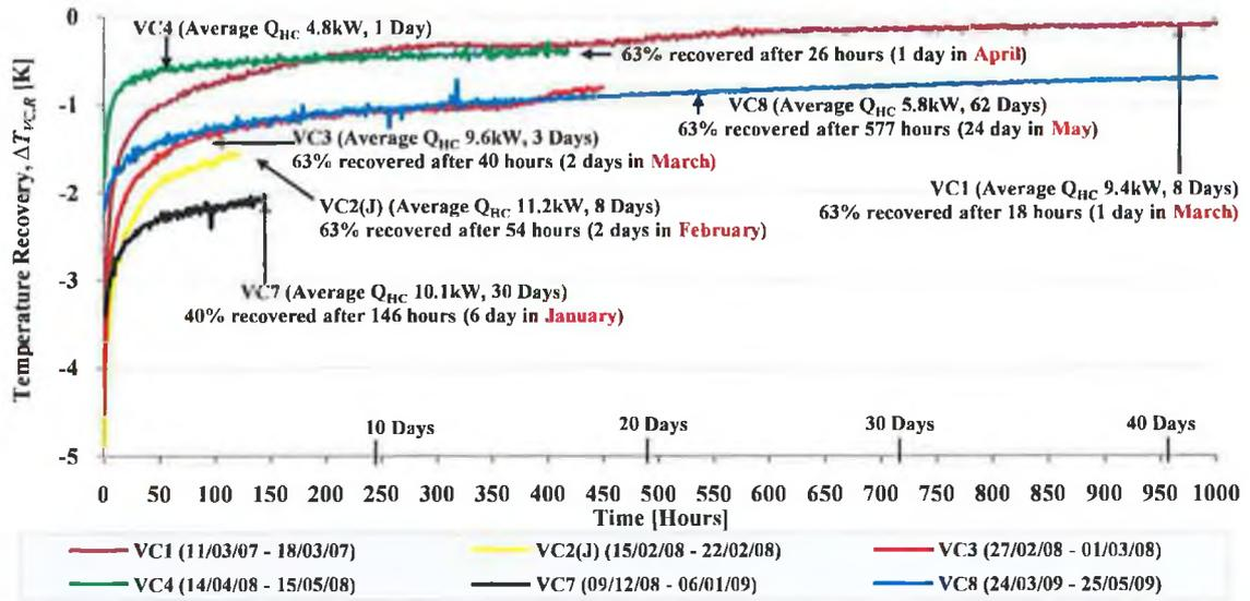
FIGURE 6.13 THERMAL RECOVERY OF THE VERTICAL COLLECTOR AT A DEPTH OF 50M AFTER TEST PERIODS VC1 TO VC8.
