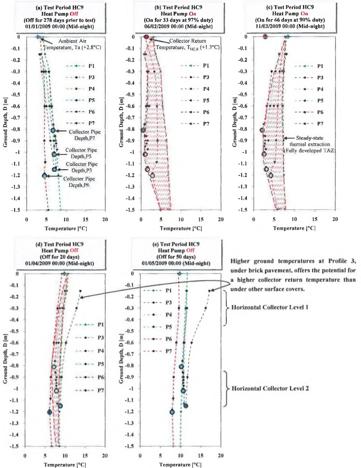
FIGURE 4.30 LONG-TERM EXPANSION AND CONTRACTION OF THE THERMALLY AFFECTED ZONE FROM TEST PERIOD HC9.
