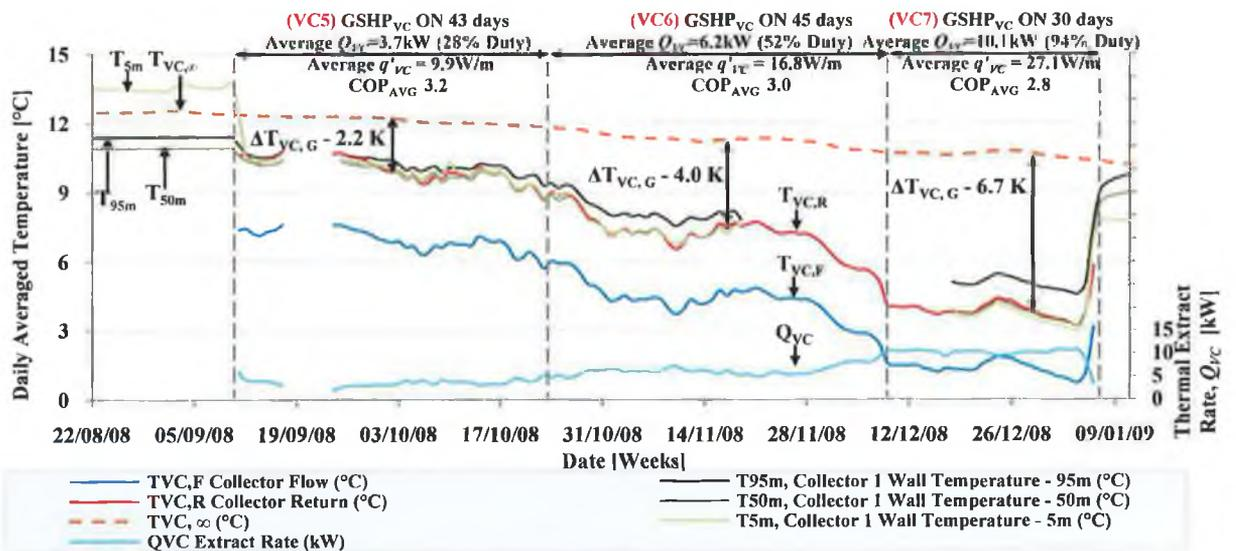
FIGURE 6.9 DAILY AVERAGED GROUND TEMPERATURE DRAWDOWN DURING THE CONSECUTIVE LOW, MODERATE AND INTENSIVE VERTICAL COLLECTOR THERMAL EXTRACTION PERIODS VC5, 6 AND 7.
