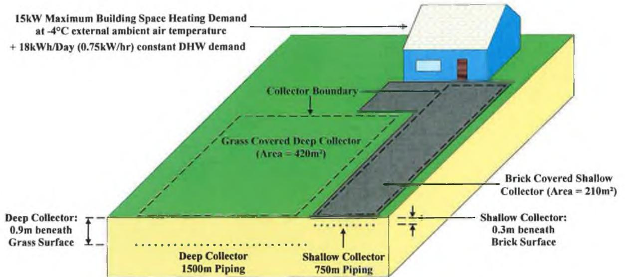
FIGURE 5.9 ALTERNATIVE, MARITIME CLIMATE SENSITIVE SPLIT LEVEL HORIZONTAL COLLECTOR DESIGN.
