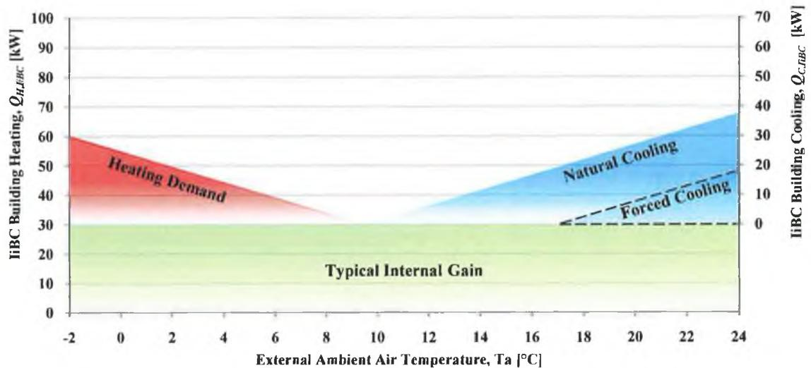
FIGURE 3.2 IIBC BUILDING DESIGN HEAT LOSS AND GAINS ANALYSIS VERSUS EXTERNAL AMBIENT AIR TEMPERATURE.
