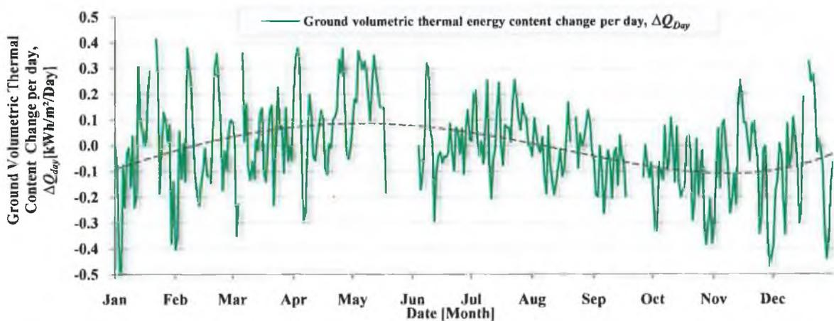
FIGURE 4.15 TOTAL CHANGE IN GROUND VOLUMETRIC THERMAL ENERGY CONTENT AT PROFILE 1 PER DAY OVER 2008.
