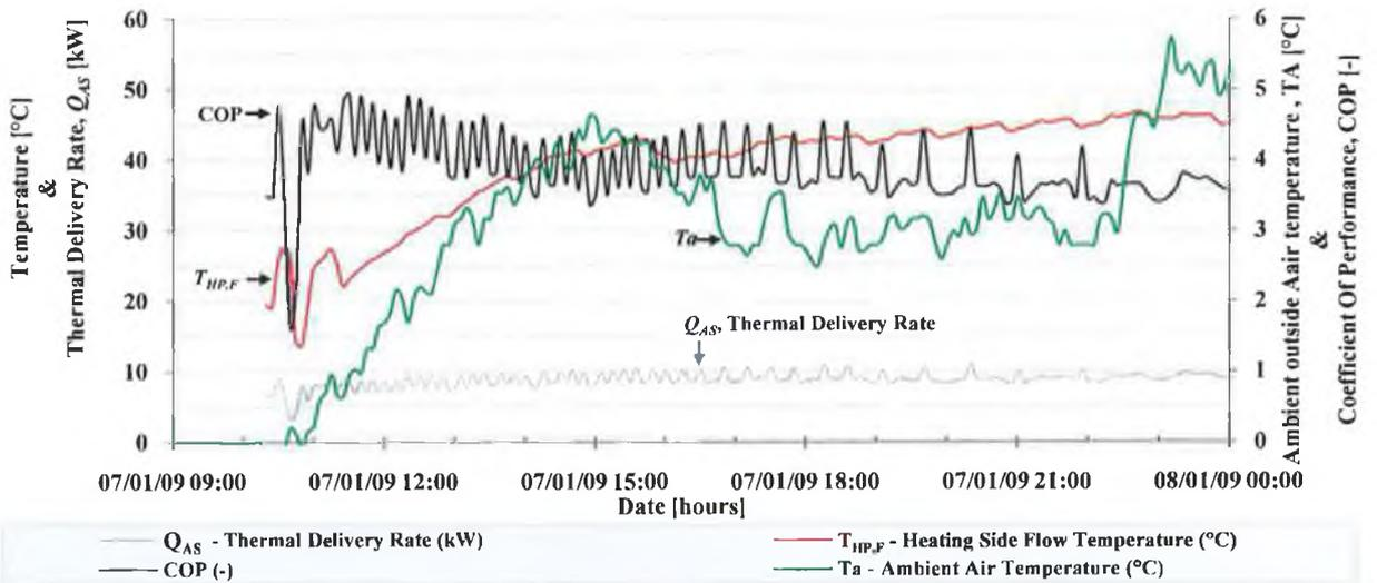
FIGURE 6.24 FIVE MINUTE RECORDING INTERVALS OF ASHP START-UP PERFORMANCE FOR TEST PERIOD AS2.
