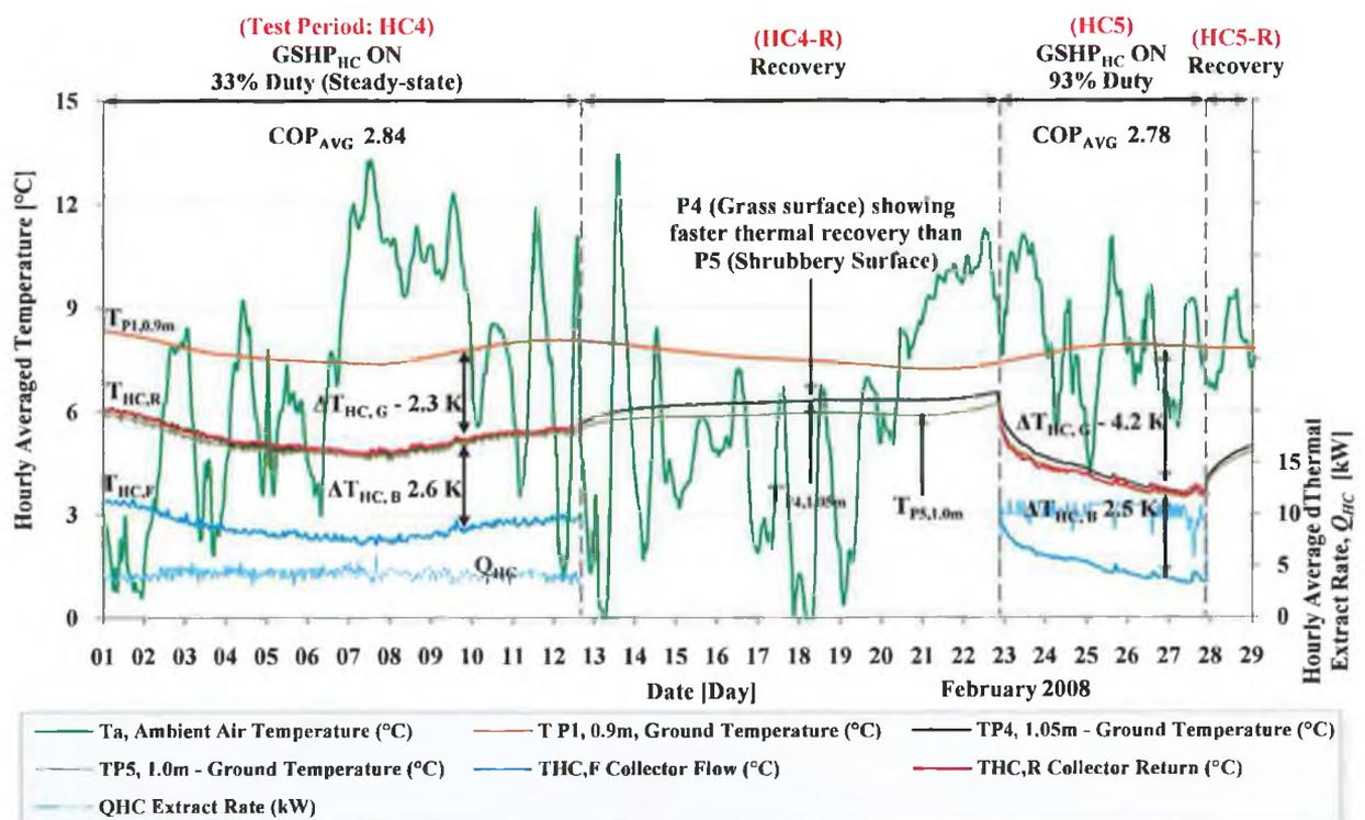
**FIGURE 4.35** DRAWDOWN AND RECOVERY OF THE GROUND TEMPERATURE IN THE COLLECTOR REGION OF THE GSHP<sub>HC</sub> DURING TEST PERIODS HC4 AND HC5.
