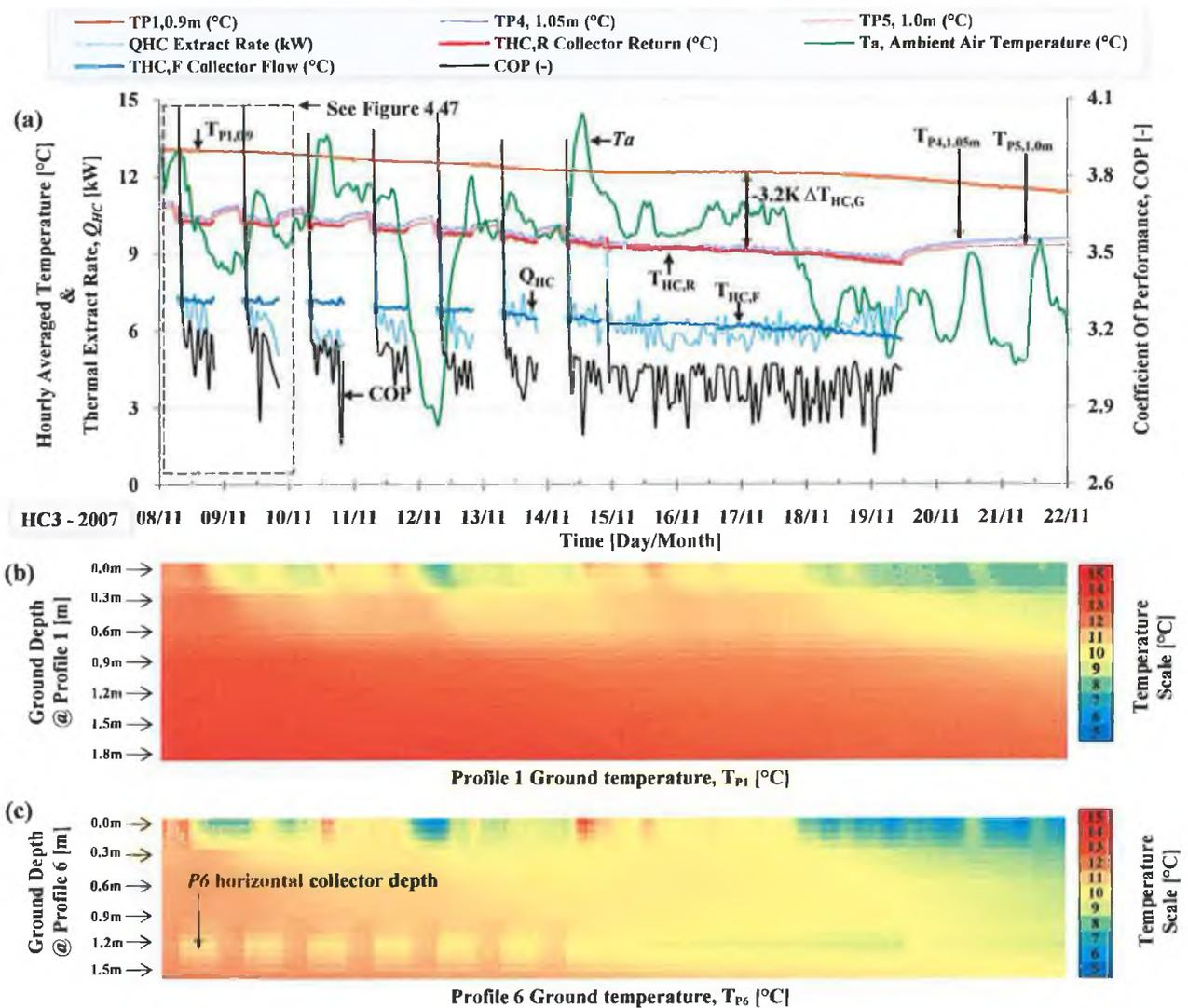
**FIGURE 4.33** (A) HOURLY AVERAGED HEAT PUMP AND COLLECTOR PERFORMANCE IN TEST PERIOD HC3, (B) PROFILE 1 3-D REFERENCE TRANSIENT TEMPERATURE MAP AND (C) PROFILE 6 3-D TRANSIENT TEMPERATURE MAP OF GROUND TEMPERATURE DRAWDOWN AND RECOVERY IN THE HORIZONTAL COLLECTOR REGION.
