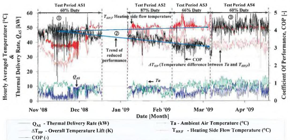
**FIGURE 6.20** TIMING OF FOUR OF THE ASHP TEST PERIODS (2008-2009) AND CORRESPONDING PERFORMANCE.
