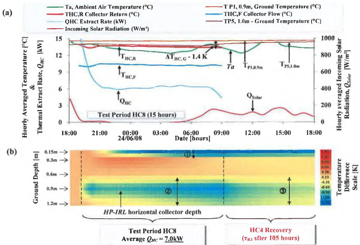
**FIGURE 4.25** (A) SHORT-TERM, MODERATE THERMAL EXTRACTION FROM HORIZONTAL COLLECTOR AND (B) TAZ AROUND THE HORIZONTAL COLLECTOR DURING TEST HC8 ESTABLISHED BY SUBTRACTING GROUND TEMPERATURES AT PROFILE 1 FROM GROUND TEMPERATURES AT PROFILE 5 (P5-P1).
