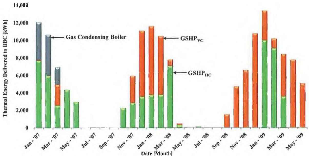
**FIGURE 3.4** RESPECTIVE CONTRIBUTIONS OF THE GSHP<sub>HC</sub>, GSHP<sub>VC</sub> & GAS HEATING SYSTEMS TO THE IIBC HEAT DEMAND PER MONTH BETWEEN JANUARY, 2007 AND JUNE, 2009.
