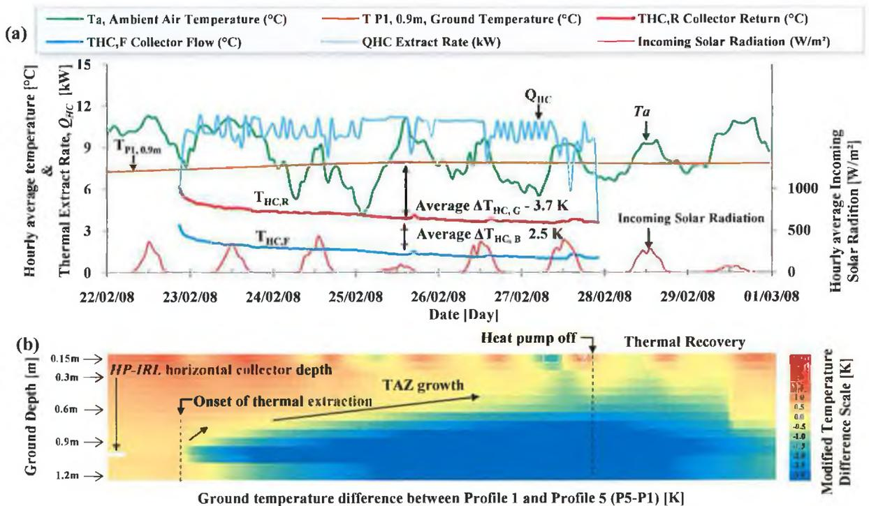
**FIGURE 4.26** (A) SHORT-TERM, INTENSIVE THERMAL EXTRACTION (93%) DURING TEST PERIOD HC5 AND (B) 3-D TEMPERATURE DIFFERENCE MAP ILLUSTRATING THE TAZ AROUND THE HORIZONTAL COLLECTOR DURING TEST HC8, ESTABLISHED BY SUBTRACTING GROUND TEMPERATURES AT PROFILE 1 FROM GROUND TEMPERATURES AT PROFILE 5 (P5-P1).
