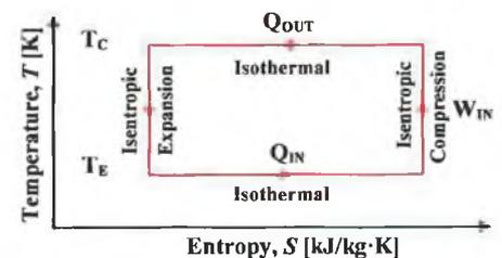
FIGURE 1.2 HEAT PUMP TEMPERATURE-ENTROPY (T-S) DIAGRAM.
