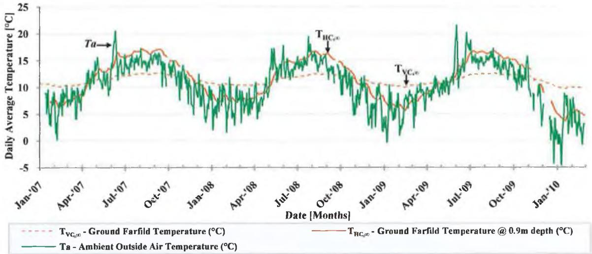
FIGURE 7.1 HEAT PUMP SOURCE TEMPERATURE COMPARISON BETWEEN JANUARY 2007 AND FEBRUARY 2010.
