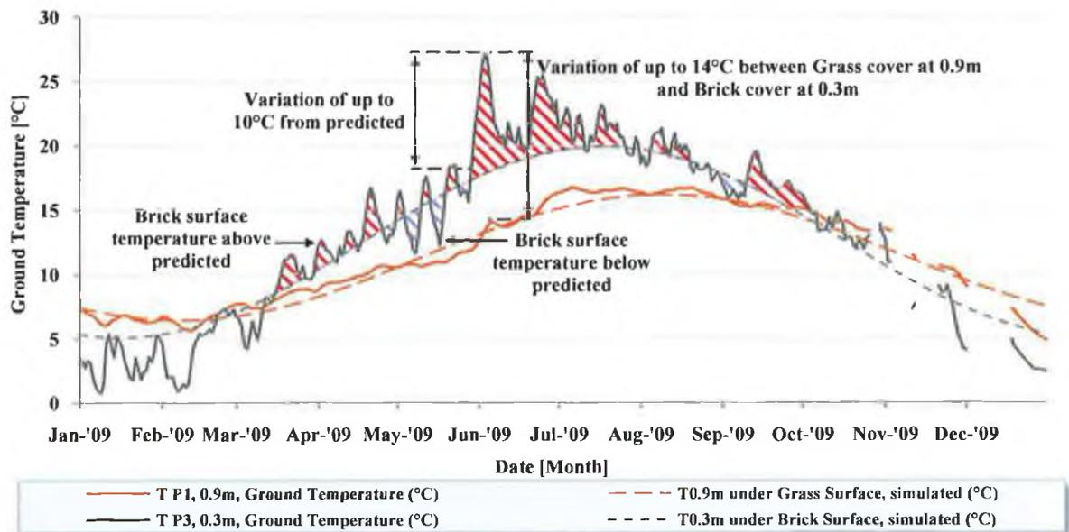
**FIGURE 5.6** DAILY AVERAGED MEASURED AND PREDICTED GROUND TEMPERATURES UNDER A GRASS AND BRICK COVERED SURFACE AT DEPTHS OF 0.3M AND 0.9M DURING 2009.
