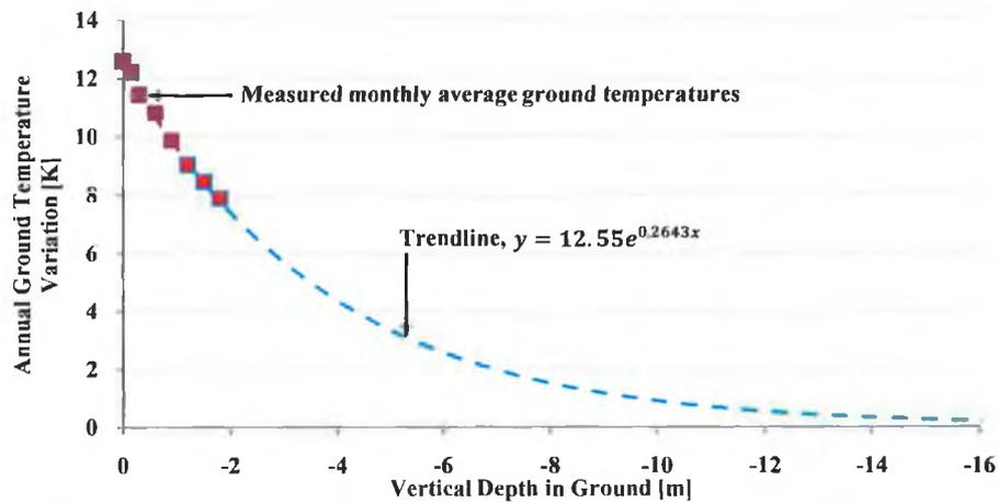
**FIGURE 6.1** EXTRAPOLATION OF MEASURED MONTHLY AVERAGED DATA TO PREDICT GROUND TEMPERATURE VARIATION FROM MEAN TO A DEPTH OF 16M IN GALWAY.
