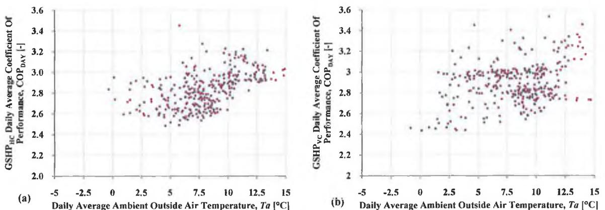
FIGURE 7.2  $COP_{DAY}$  VALUES FOR (A) GSHP<sub>HC</sub> AND (B) GSHP<sub>VC</sub> SYSTEMS OVER THE TOTAL TEST PERIOD FROM THE 1<sup>ST</sup> OF JANUARY 2007 TO THE 1<sup>ST</sup> OF MARCH 2010.
