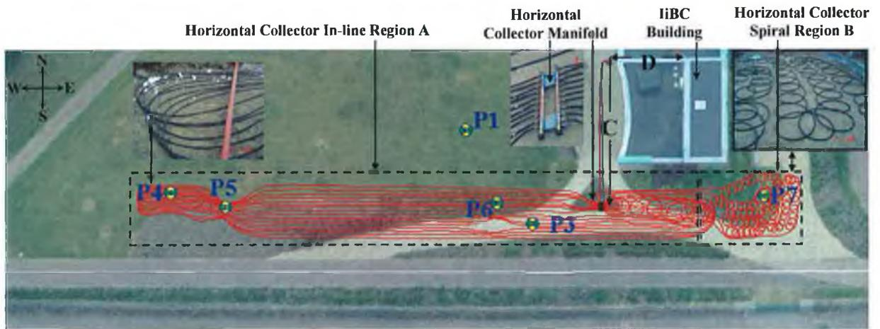
**FIGURE 3.16** AERIAL PHOTOGRAPH OF HORIZONTAL COLLECTOR REGION, UPON WHICH THE ACTUAL COLLECTOR CONFIGURATION HAS BEEN SUPERIMPOSED FROM PHOTOS TAKEN DURING INSTALLATION.
