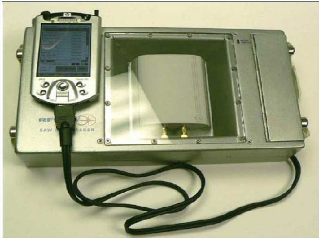
Figure 8 - NASA version of the SAW 704 reader with PDA (source: NASA)
