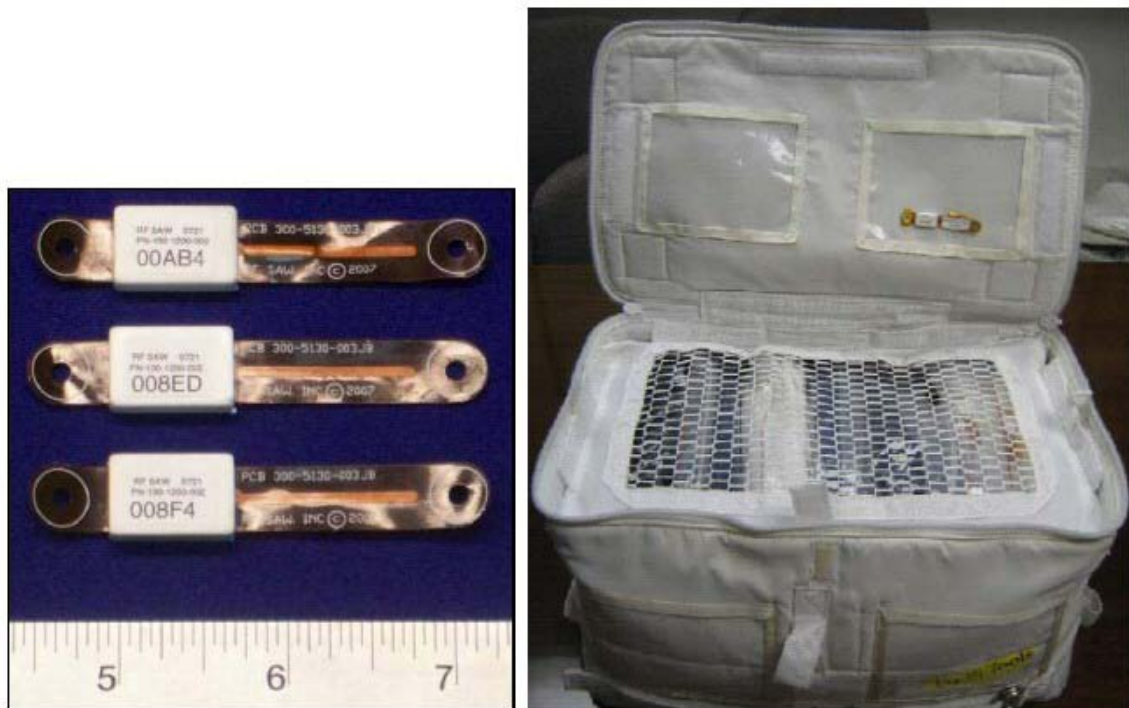
Figure 7 - SAW RFID tags and tagged flight-bag (source: NASA)
