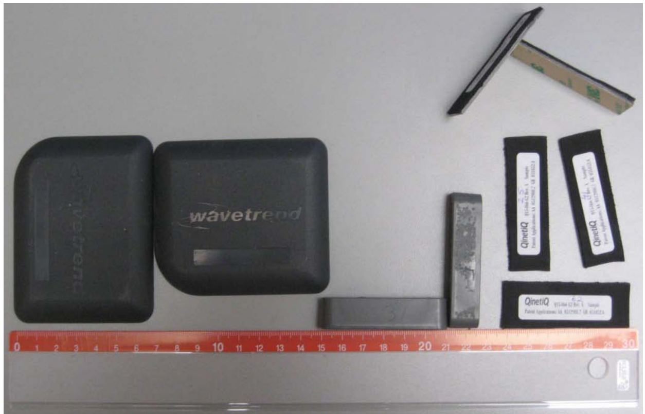
Figure 3 - Mixture of active and passive tags used in the project
