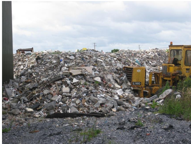
Picture 7.14 Concrete/ rubble waste holding area
