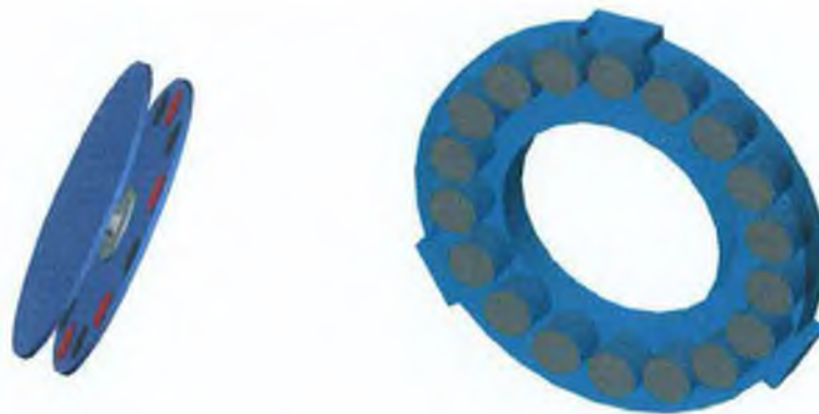
Fig 6.11 Generator components - rotor and stator
