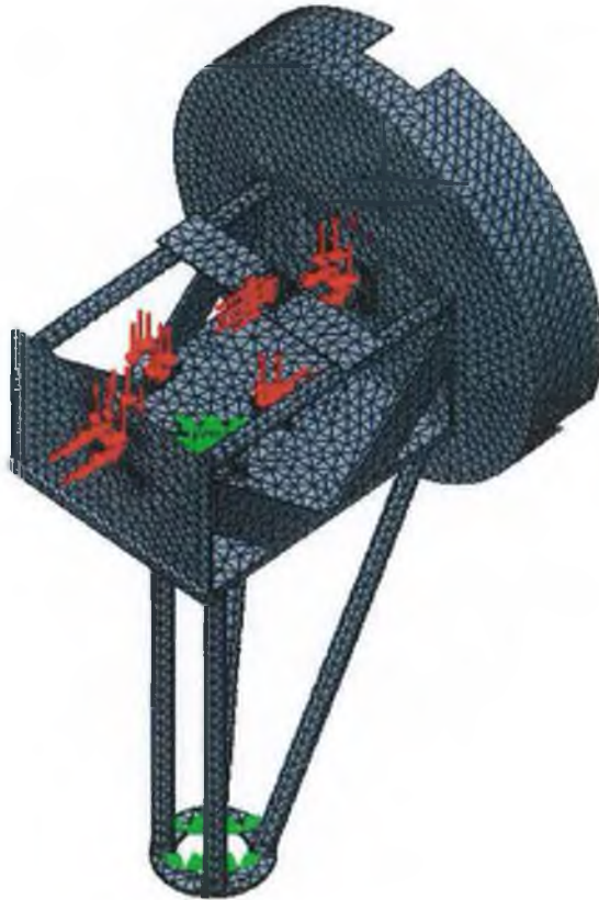
Fig. 7.5 Meshed model of the top structure for finite element analysis
