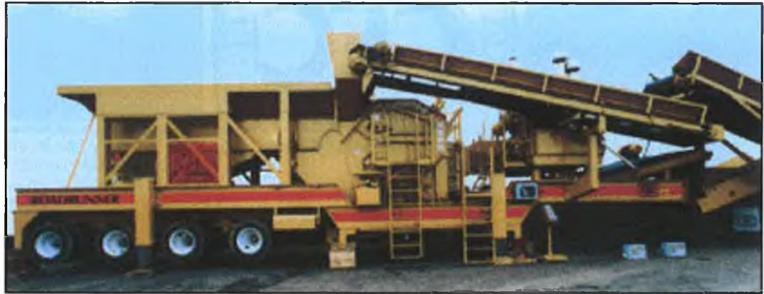
Photograph 5.5 A 'grizzly' screen incorporated into a mobile crushing system (Construction Equipment Co., USA)
