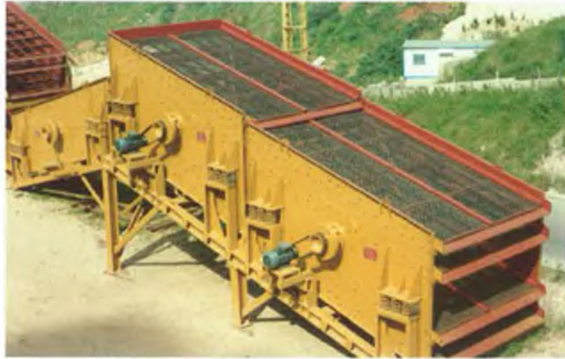
Photograph 5.7 A vibratory screen (Armico Ltd., Lebanon)
