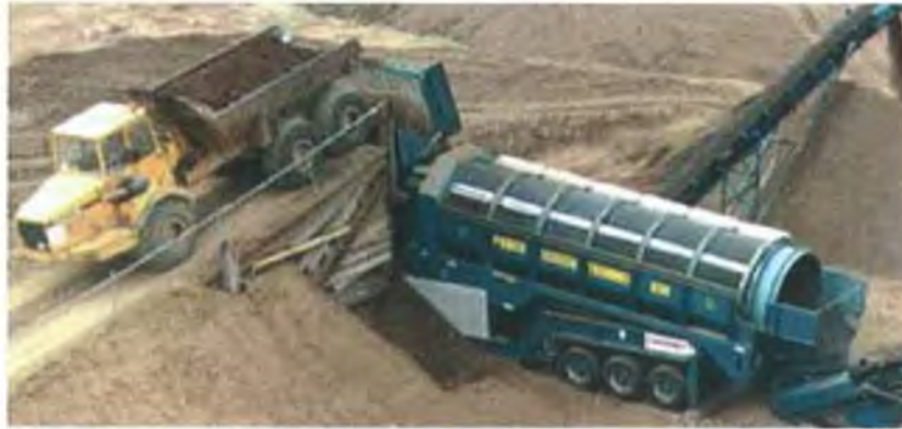
Photograph 5.6 A trommel in operation (Powerscreen Ltd., U.K.)
