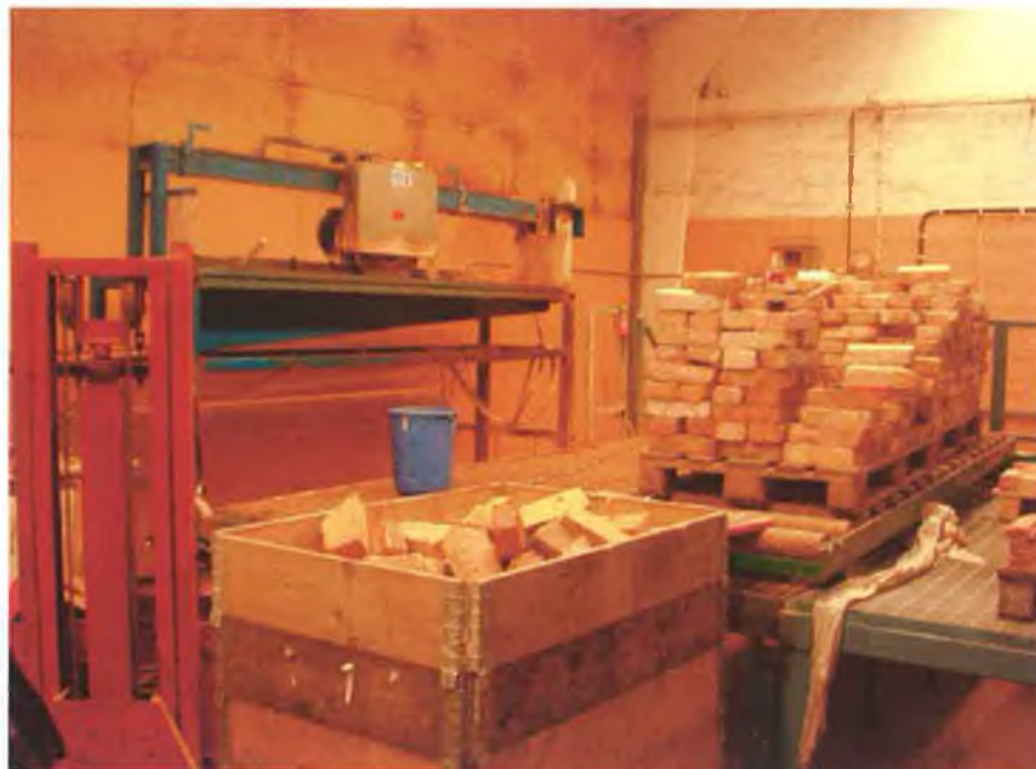
Photograph 6.19 Recycling/restoration of bricks at the Malmo Aterbyggdena store
