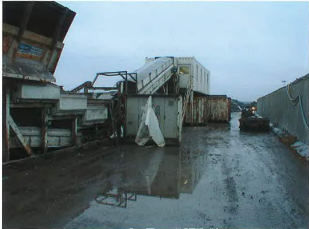
Photograph 5.1 Heavy-duty steel-apron conveyor in operation (Copenhagen Recycling Centre, Denmark)
