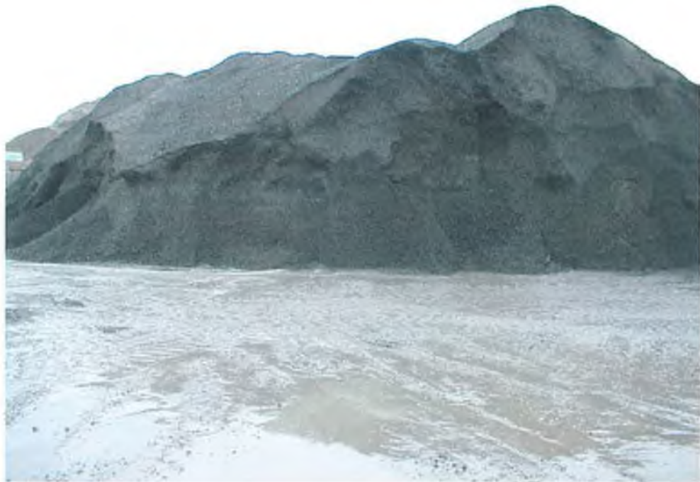
Photograph 6.13 Crushed asphalt/concrete stored adjacent to the processing operations at the Copenhagen Recycling Centre
