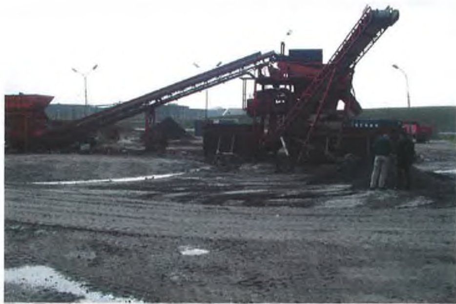
Photograph 6.22 Processing of incinerator ash (slag) at the Spillepeng Landfill
