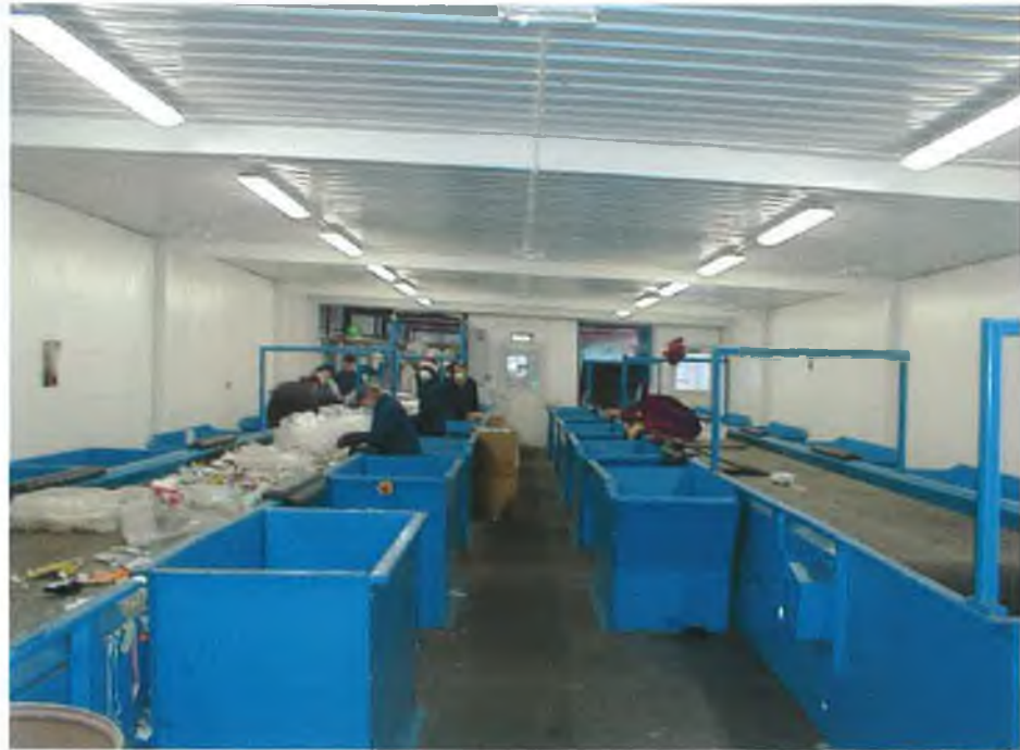
Photograph 5.9 Manual Picking Station in operation at the Barna Waste facility in Galway
