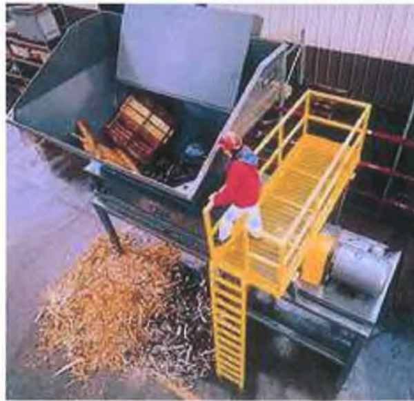
Photograph 5.4 A rotary shear shredder in operation
