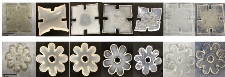
Figure 13. The appearance of the 4D printed jigsaw and flower samples sample at times (from left): 0 h; 6 h; 24 h; 72 h; 168 h; 240 h; 408 h.
