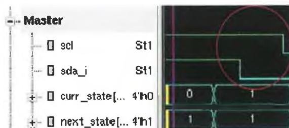
Figure 6.14 Generating Start condition
