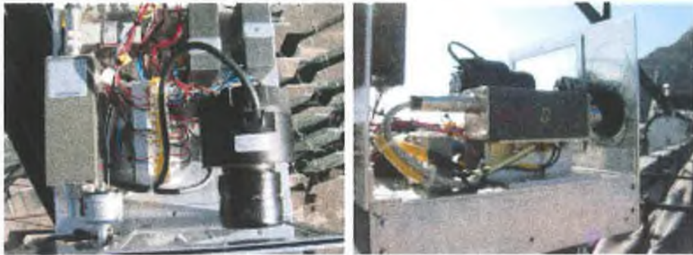
Figure 2.2: Two views of the CCD camera and FIR pyrometer in their protective housing (with the top cover removed for purpose of photograph).
