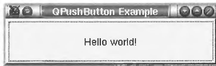
Figure 3.5: A screen-shot of a basic Qt widget with only one pushbutton, entitled “Hello world!”.
