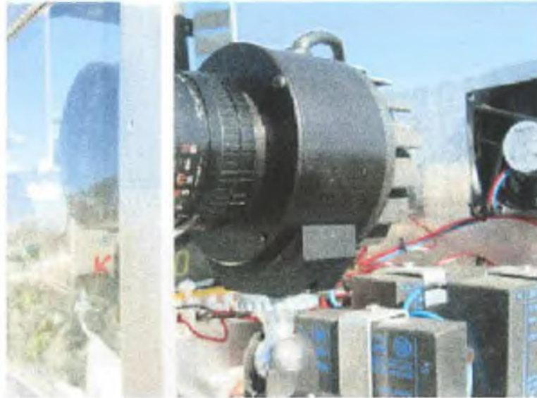
Figure 2.8: The focused CCD camera mounted in its housing on one of the side arms of the Whipple ten metre telescope. The housing cover was removed for the purpose of illustration.
