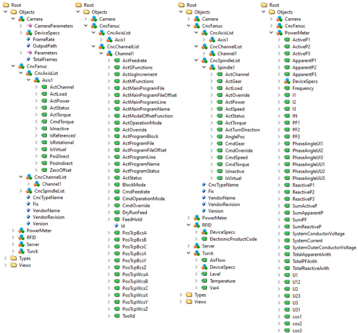
Fig. 2. Four views of the same CNC OPC UA server address space, with different nodes expanded in each view, obtained using UA expert.
