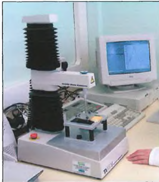
Figure 4. The TAXT2i Texture Analyser used for measuring springiness in fish portions
