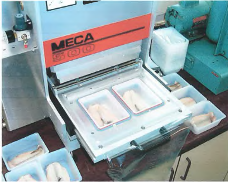
Figure 3. Modified atmosphere packaging of whiting fillets in plastic trays using the Mecapac 500 MAP packaging machine
