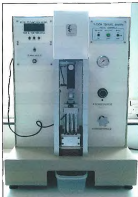
Figure 5. The T-2000 Texture System with Kramer shear cell attached
