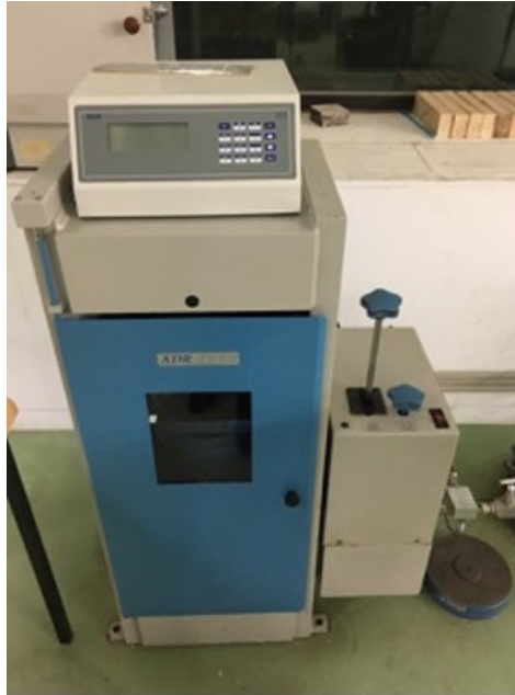
Figure 3.12 Equipment used to determine the compressive strength of specimens..
