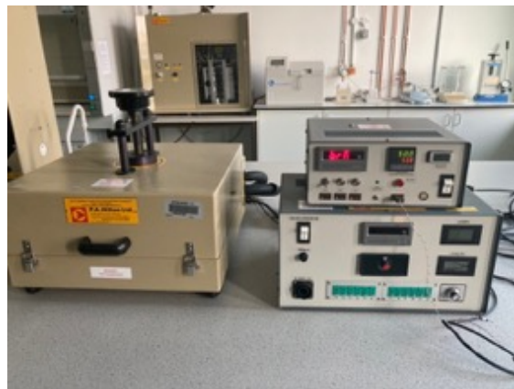
Figure 3.17 –Equipment used to measure thermal conductivity.
