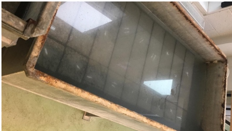
Figure 3.10 Concrete curing tank set at (21 \pm 1)^\circ\text{C} .
