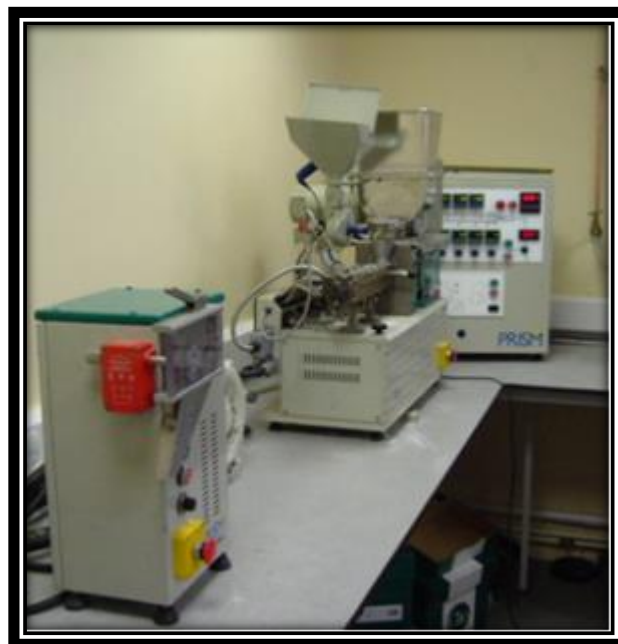
Figure 19. The Prism™ twin screw 15:1 L/D ratio extruder used in this study.
