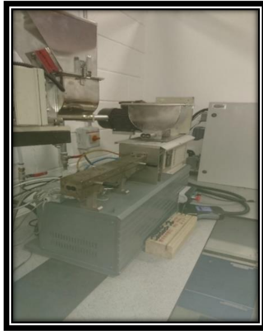
Figure 17. The Prism TM twin screw 25:1 length to diameter (L/D) ratio extruder used in this study.
