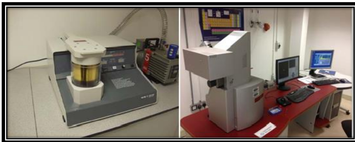
Figure 23. Mira scanning electron microscope (SEM) (left hand side) and Bal-Tec SCD005 sputter coater (right hand side).
