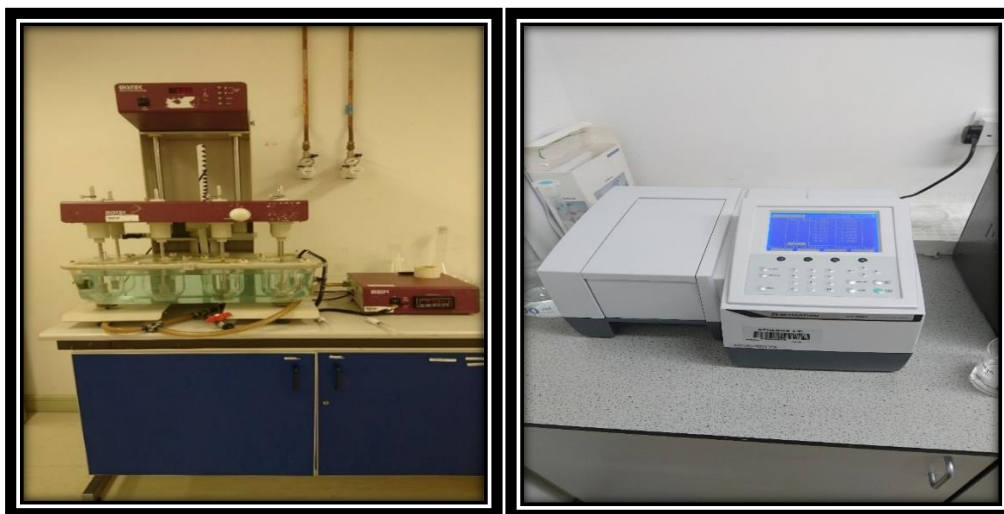
Figure 24. Distek 50947 dissolution apparatus (left hand side) and UV-1280 ultraviolet (UV)-Vis (UV) Spectrophotometer (Right hand side).
