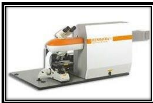
Figure 21. Renishaw inVia Raman confocal microscope attached to a motorized stage.
