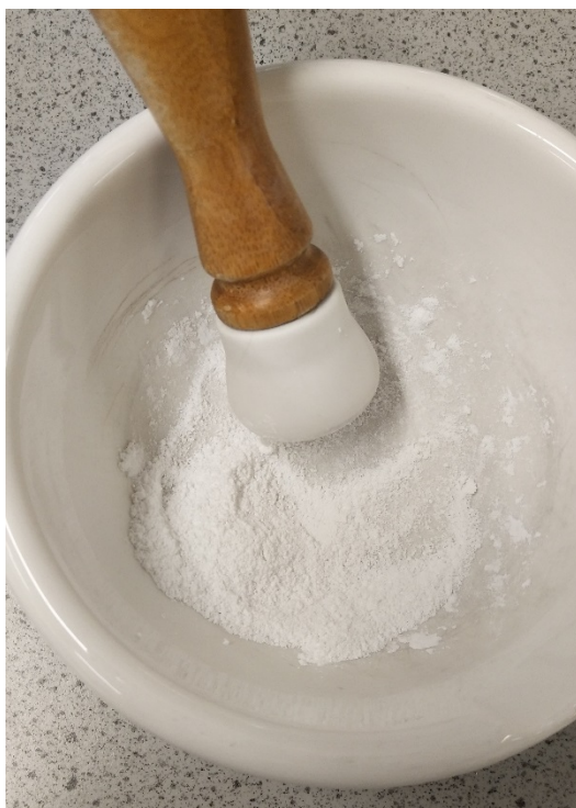
Figure 2.1 Fluorapatite (FAp) powder prepared through chemical substitution method.
