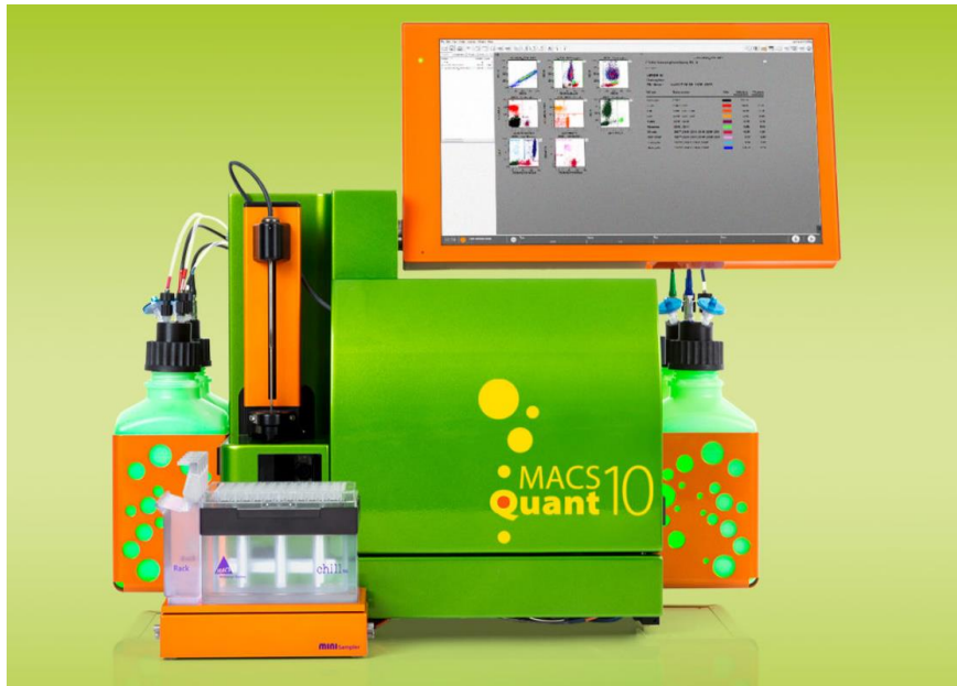
Figure 2 Flow cytometer used for data analysis of cells and spores. Image referenced from miltenyibiotec. https://www.miltenyibiotec.com/US-en/products/macsqunt-analyzer-10.html#gref
