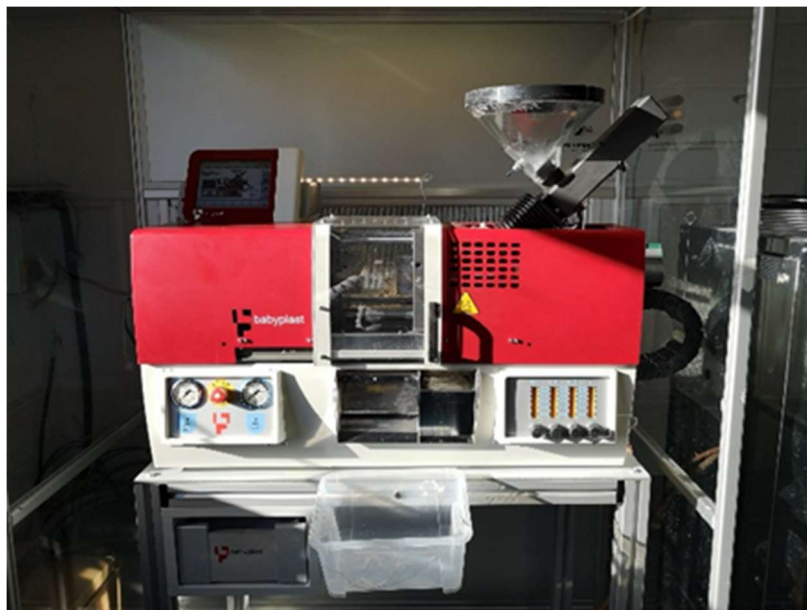
Figure 3-8 Babyplast IMM utilized in IM processing.
