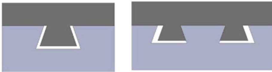
Figure 2-13 Mechanical Interlocking employed in the combination of AM and cutting, reproduced from (Weflen & Frank, 2021).
