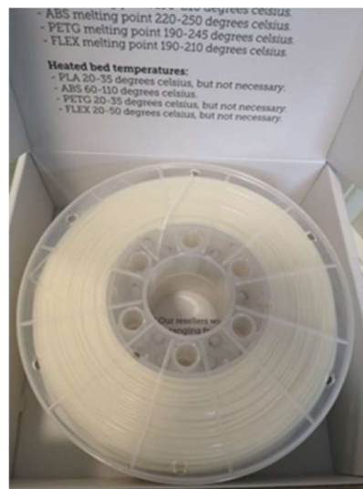
Figure 3-1 Filament utilized in the fabrication of ABS printed samples/inserts.
