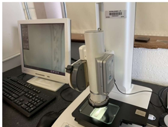
Figure 3-11 Nikon ShuttlePix P-MFSC observing the specimen.
