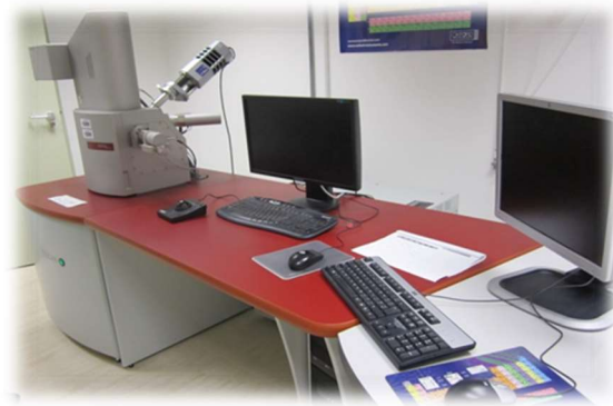
Figure 3-12 Mira FE scanning electron microscopy utilized in the study.
