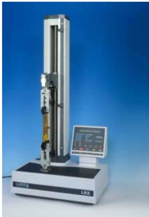
Figure 3-9 LRX single column, bench mounted materials testing system machine utilized for test.
