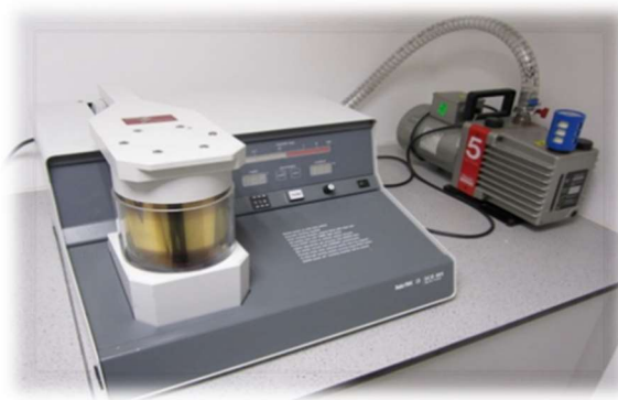
Figure 3-13 Baltec SCD 005 Sputter Coater utilized before SEM observation.
