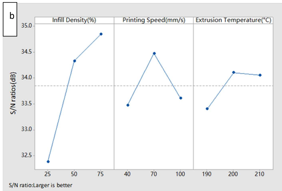
Figure 7-4 Plots of the main effects of the parameters used in PLA pieces on the (a) tensile strength and (b) S/N ratio of the tensile strength, where the dashed line indicates the average result.
