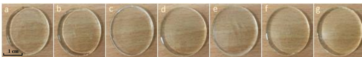
Figure 3-3 PNVCL xerogels fabricated using different concentrations of Irgacure 2959 initiator: a) 0.1 wt%; b) 0.2 wt%; c) 0.5 wt%; d) 1 wt%; e) 2 wt%; f) 3 wt%; g) 5 wt%.
