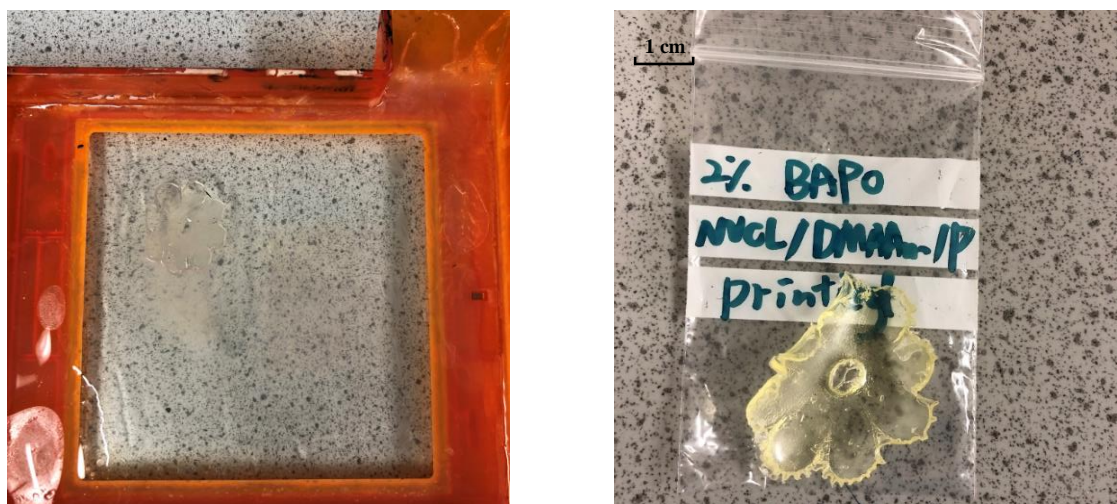
Figure 3-43 (L) the BAPO sample printed flower shape model stuck on the resin-filling tank; (R) flower-shaped sample printed with 2 wt% BAPO resin.
