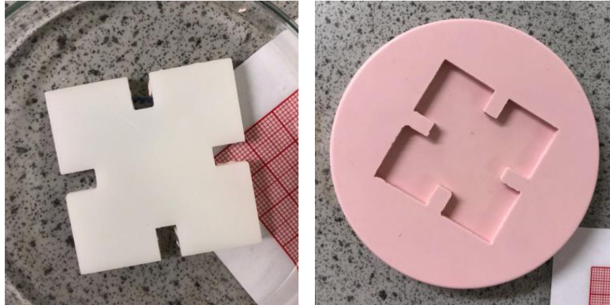
Figure 2-2 (L) The printed jigsaw shape prototype & (R) the jigsaw type silicone mould.
