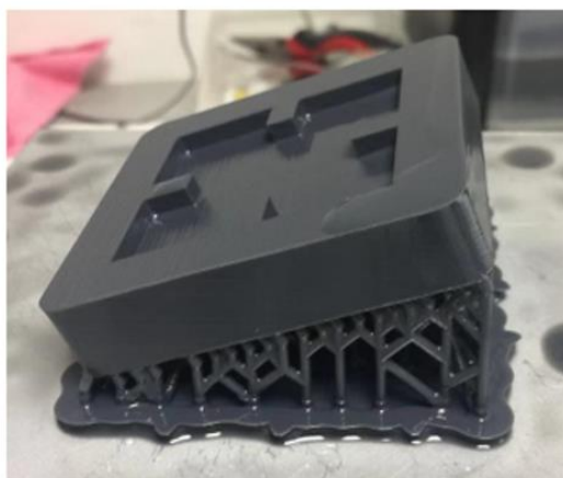
Figure 3-37 Mould printed using Form 2 3D printer.
