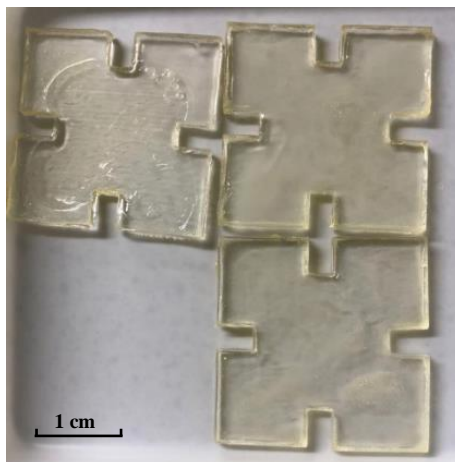
Figure 3-39 The puzzle shape samples developed using the UV curing chamber.
