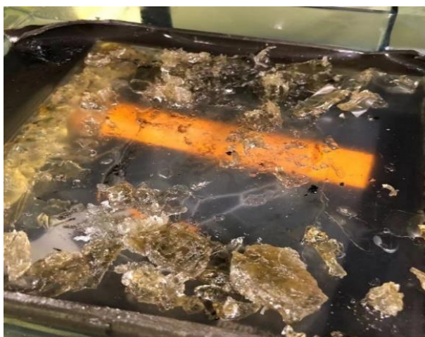
Figure 3-42 Recrystallisation of NVCL based solution occurs on the printer resin tank.
