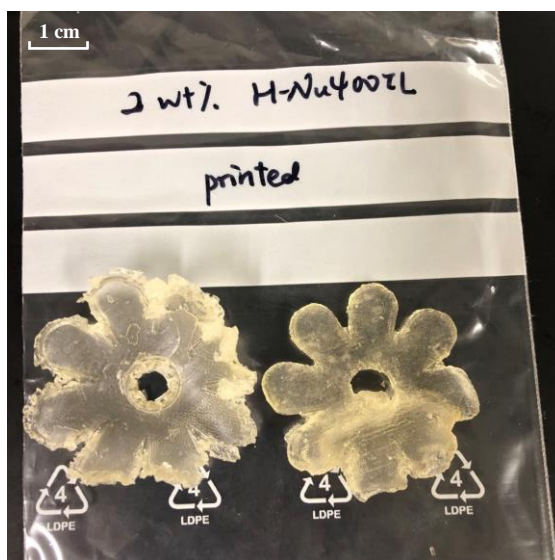
Figure 3-44 Flower-shaped parts printed using 2 wt% H-Nu 400IL resin.
