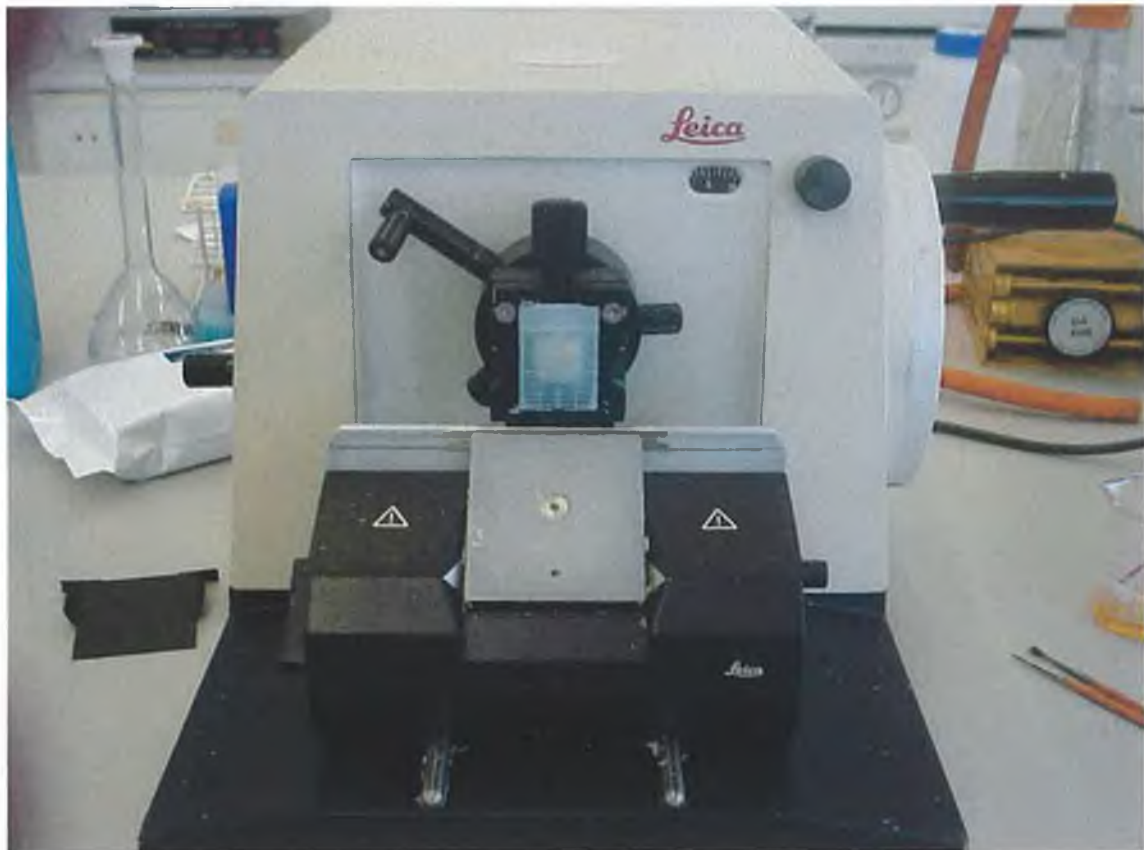
Plate 17. Leica Jung RM2025 ® rotary microtome used to section gonadal tissue at approximately 5-8 \mu m in thickness.
