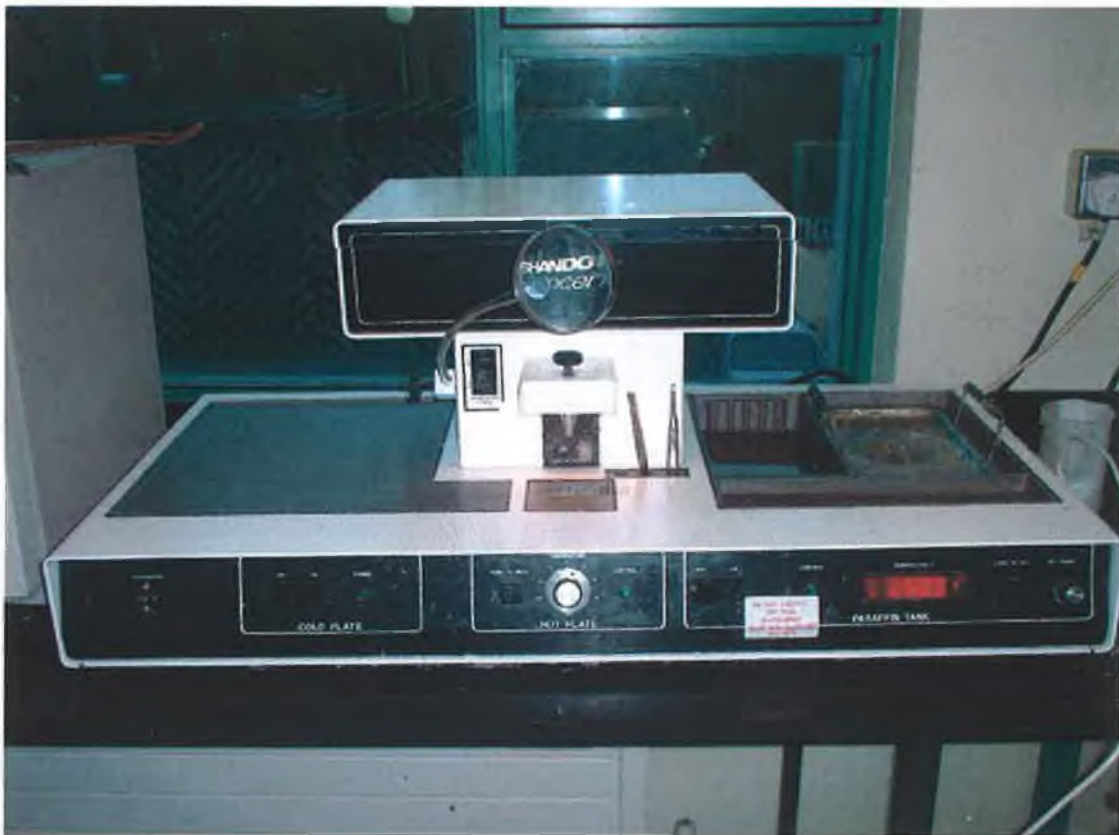
Plate 16. Shandon Histocentre ® used to block out the tissue cassettes into wax moulds.
