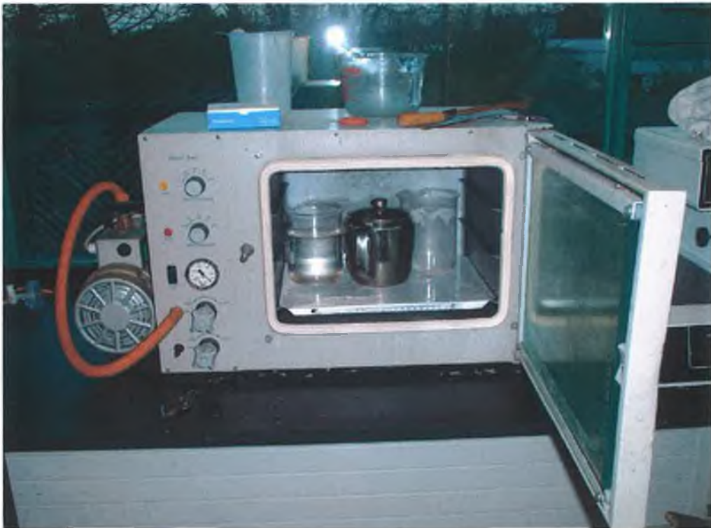
Plate 15. Gallenkamp ® vacuum oven used to fully impregnate tissue samples with paraffin wax at 600mm Hg for 30 minutes.
