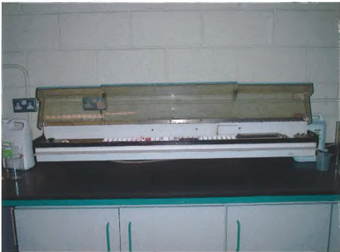
Plate 18. Shandon Linistain GLX ® stainer used to stain the sectioned gonadal tissue with a haemotoxlylin and eosin stain.
