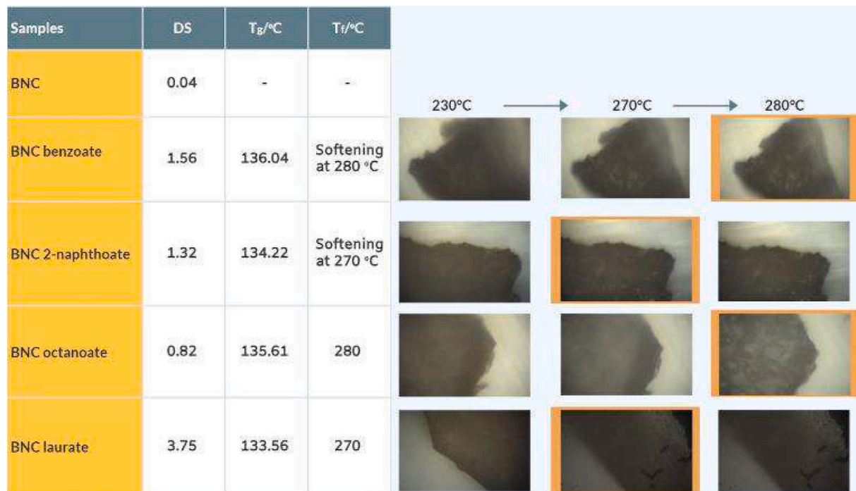
Fig. 9. Degree of substitution for bacterial nanocellulose (BNC) derivatives and their morphology under examined temperatures.
