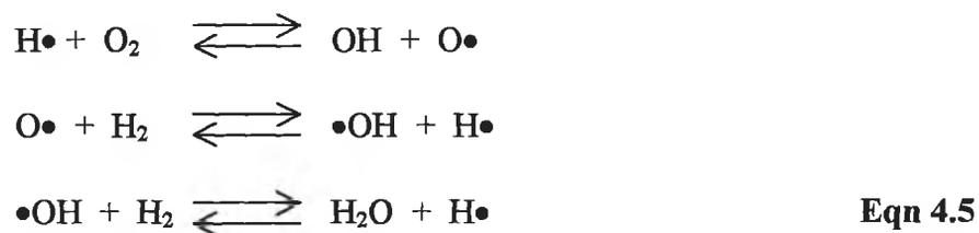
In the presence of the excess hydrogen it can be assumed that only OH and H radicals are formed and in quantities corresponding to the total amount of oxygen. The concentration of H radicals is several orders of magnitude larger than that of the OH radicals. Atomisation is via a two step mechanism with the predominating H radicals. Corresponding reactions with •OH radicals, because of their low concentration are considered negligible. The recombination reaction must also be taken into account.
