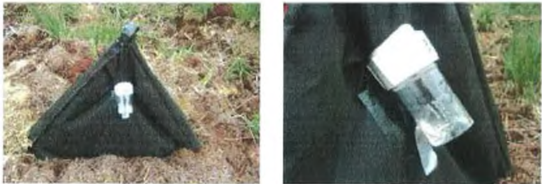
Figure 3.1. Emergence trap design.
