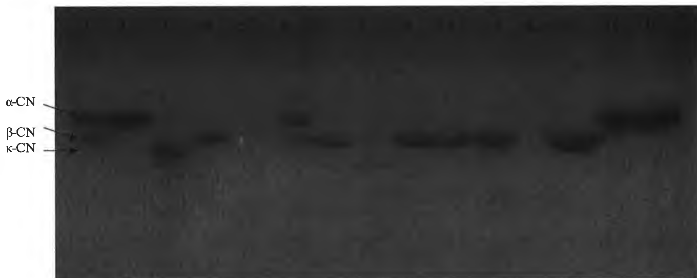
Figure 2.10. The urea-PAGE profiles of the samples obtained following the purification of \beta -casein from acid caseinate using Protocol 4.
