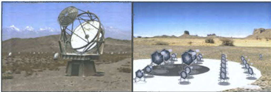
Figure 7.3 The next generation of atmospheric Cherenkov telescopes. Left: Proposed AGIS telescopes. Right: A possible design of CTA, using different sized telescopes throughout the array. Large mirrors in the centre collect enough light to catch dim showers from low-energy gamma rays. To collect large statistics at high energies, where particles are rare but the associated showers are bright, smaller mirrors cover an area of a few square kilometres (CTA Consortium 2010).
