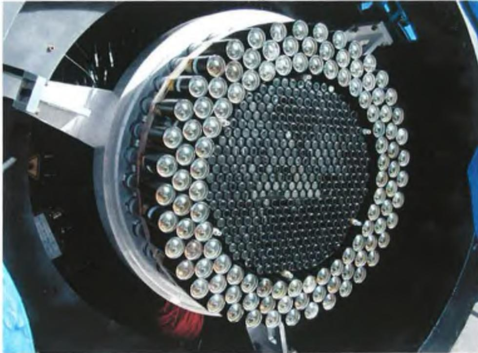
Figure 3.3: The Whipple camera with 490 photomultiplier tubes.
