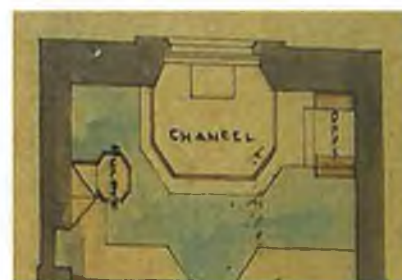
Fig. 138. Detail from Welland’s drawings for alterations to the Chancel, with pulpit on right and readers desk to the left. The altar is now back under the east window.
