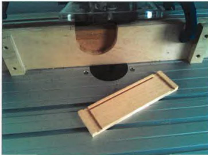
FIGURE 4.13 LONG SIDE STOPPED GROOVE ON THE TABLE ROUTER
