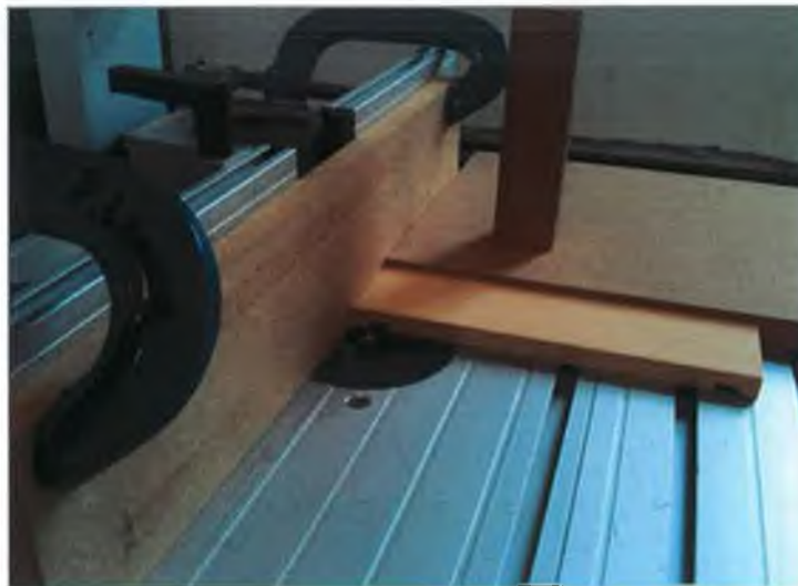
FIGURE 4.12 LONG SIDE HOUSING ON THE TABLE ROUTER
