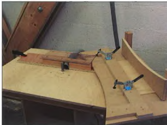
FIGURE 4.29 CONCAVE SHELF JIG ON THE TABLE ROUTER
