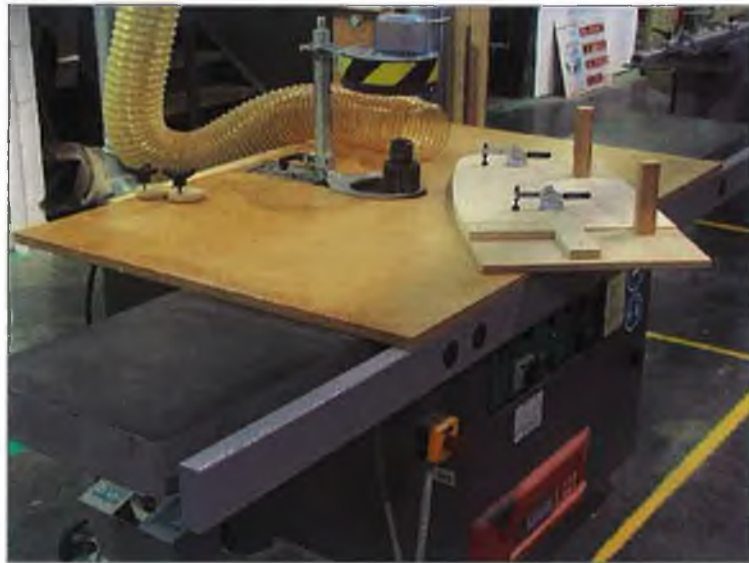
FIGURE 4.27 JIG TO PRODUCE GABLE ON THE SPINDLE MOULDER
