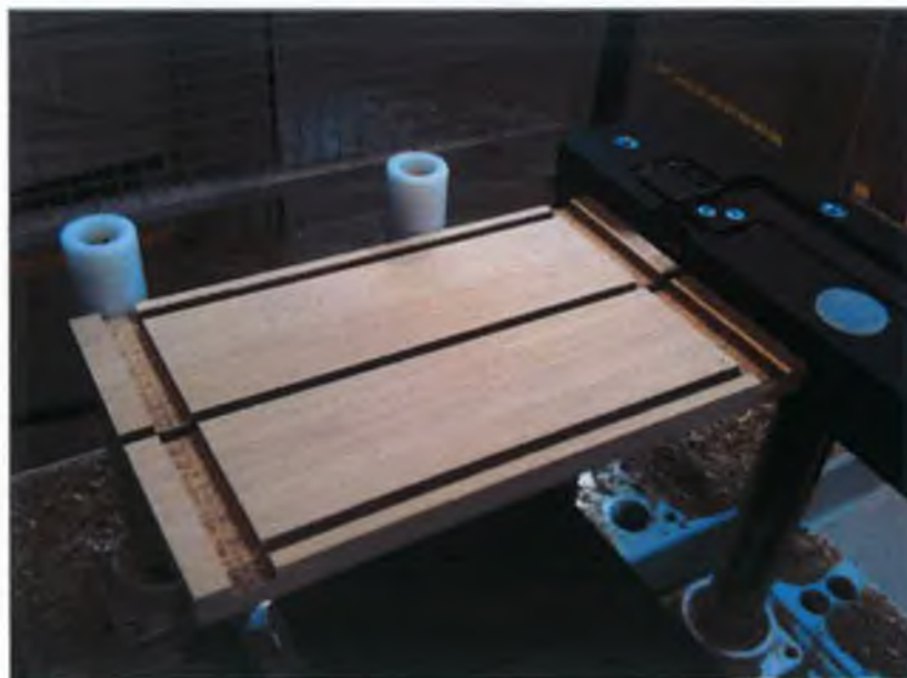
FIGURE 4.8 LONG SIDES ON THE WEEKE CNC
