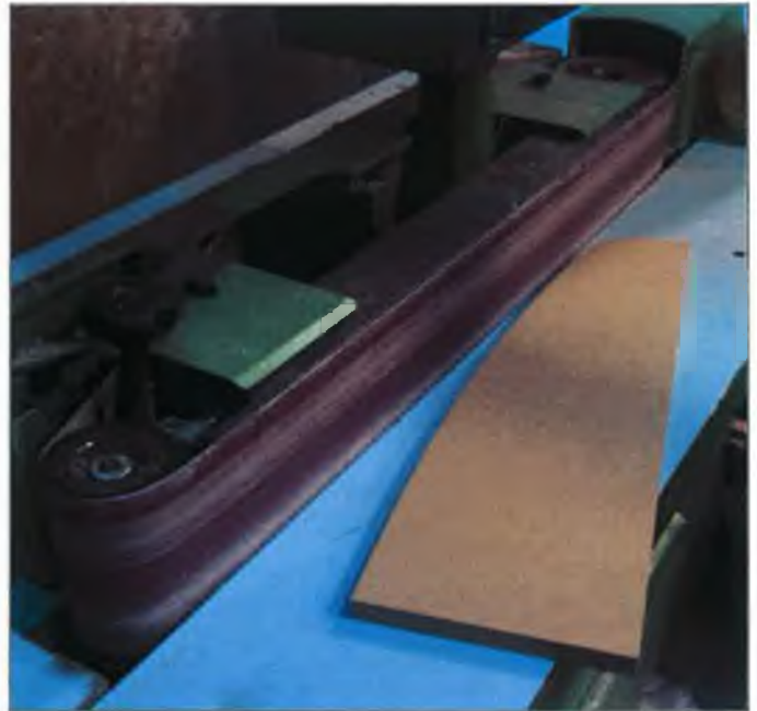
FIGURE 4.23 EDGE BEING CLEANED ON VERTICAL SANDER
