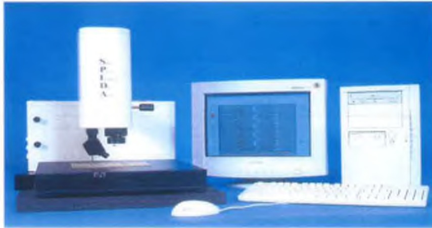
Figure 3.1 SPIDA machine for automatic solder paste height measurement and volume calculation
