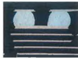
Figure 4.3 Solder joint cross section
