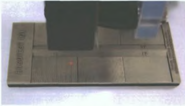
Figure 4.3: Evaluating measurement error of system using Rugotest surface comparators
